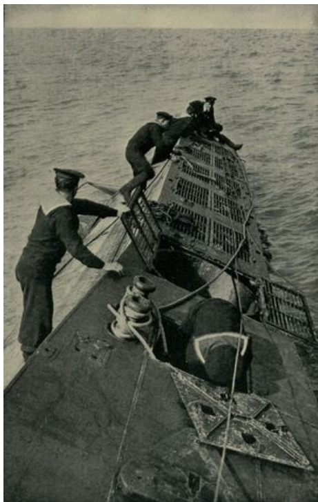
British sailors and officers boarding the captured U-C-5 German mine-laying submarine. The open grating shows one of the openings through which mines are laid.
