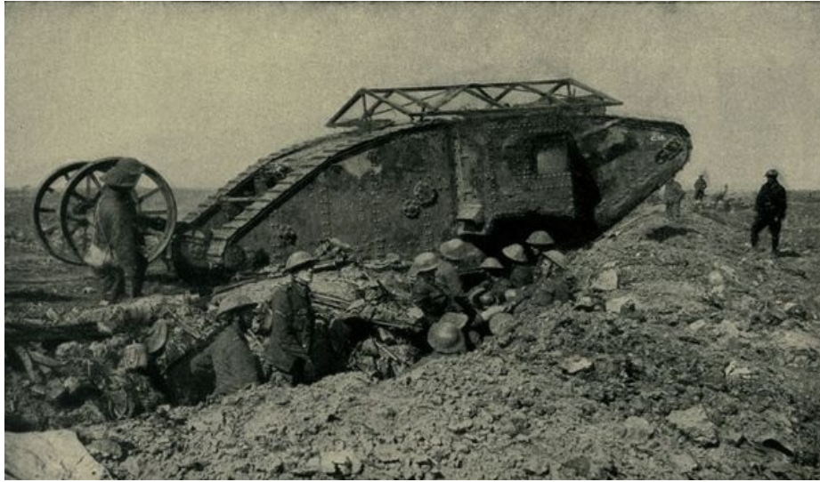
One of the strange armoured automobiles or "tanks" with which the British surprised the Germans in September, 1916. Their caterpillar trucks and peculiar form make it possible for them to advance easily over obstructions and trenches.
