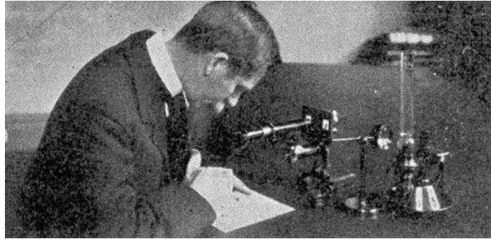
FIG. 6.—Microscope in position for drawing objects.
