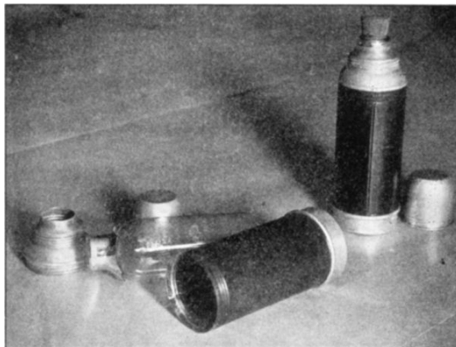
FIG. 61. How a thermos bottle is made. Notice the double layer of glass in the broken one.
