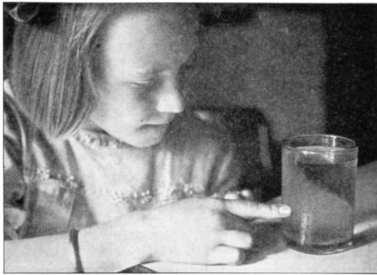
FIG. 159. The glass does not leak; the moisture on it comes from the air.
