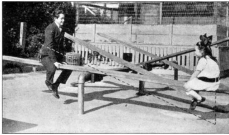
FIG. 26. The little girl raises the big boy, but in doing it she moves twice as far as he does.
