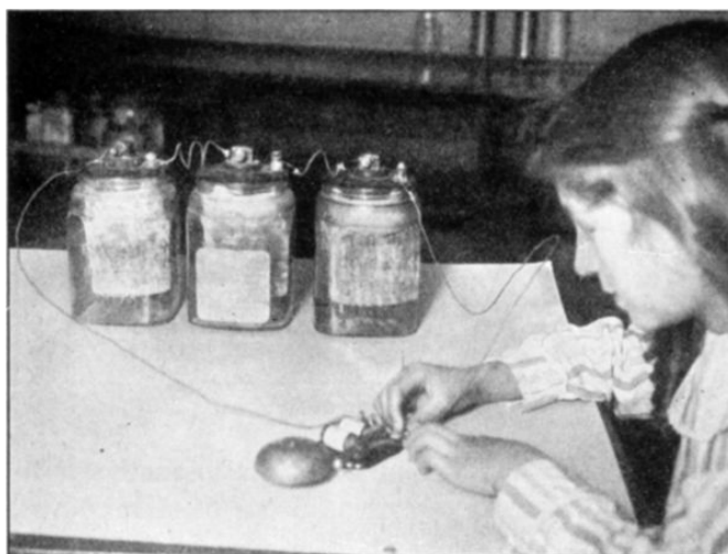
FIG. 111. A wet battery of three cells connected to ring a bell.
