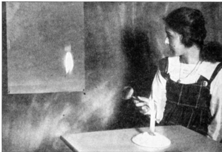
FIG. 71. The reading glass is a lens which focuses the light from the candle flame and forms an image.
