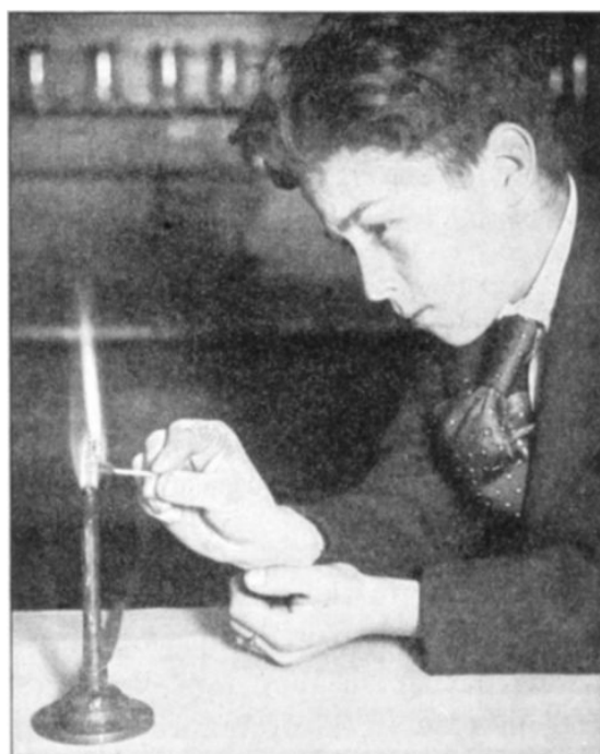
Fig. 172. The part of the match in the middle of the flame does not burn.
