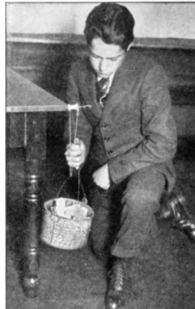
FIG. 33. With this arrangement the pail travels more slowly than the hand. Will it seem heavier or lighter than with the arrangement shown in Figure 32?
