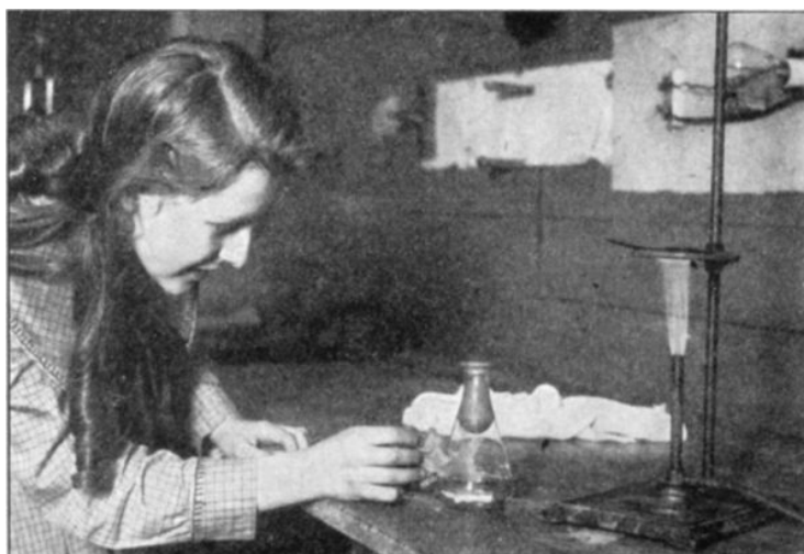
FIG. 53. As the steam condenses and leaves a vacuum, the air pressure forces the balloon into the flask.
