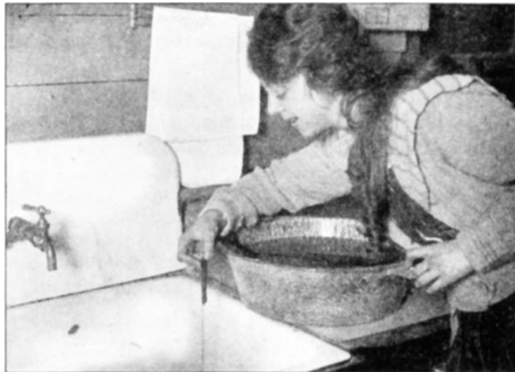
FIG. 8. A siphon. The air pushes the water over the side of the pan.
