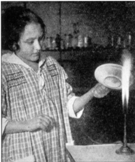
FIG. 168. The Bunsen burner smokes when the air holes are closed.
