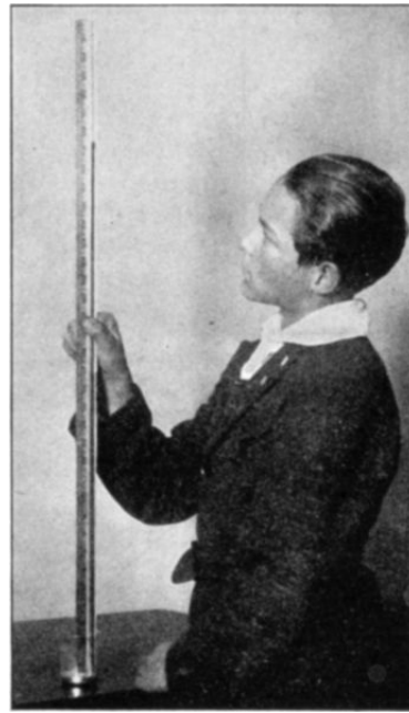
FIG. 154. Finding the pressure of the air by measuring the height of the mercury in the tube.
