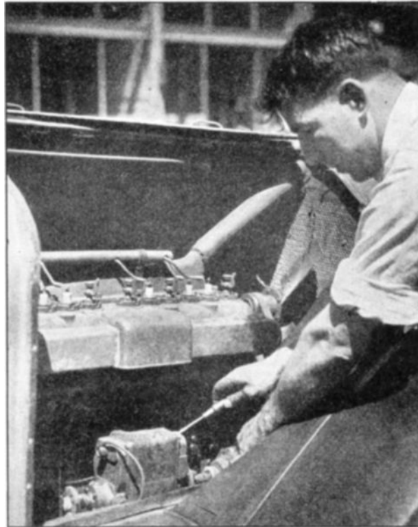
FIG. 118. The magneto in an automobile is a small dynamo.
