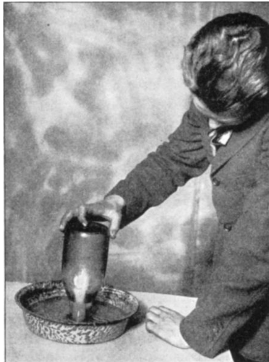
FIG. 167. The water rises in the bottle after the burning candle uses up the oxygen.
