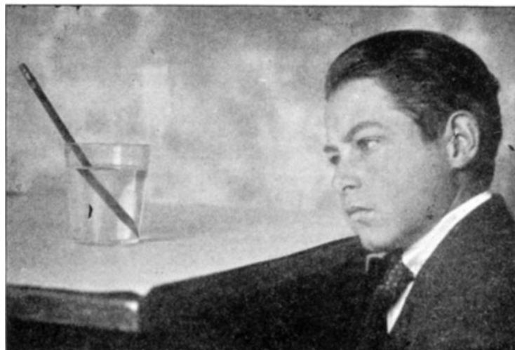
FIG. 67. The bending of the light by the water in the glass causes the pencil to look broken.
