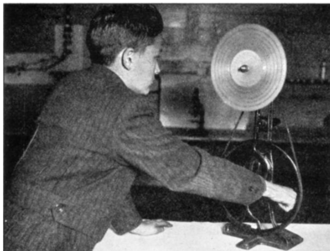
FIG. 92. When the wheel is rapidly whirled the colors blend to make white.
