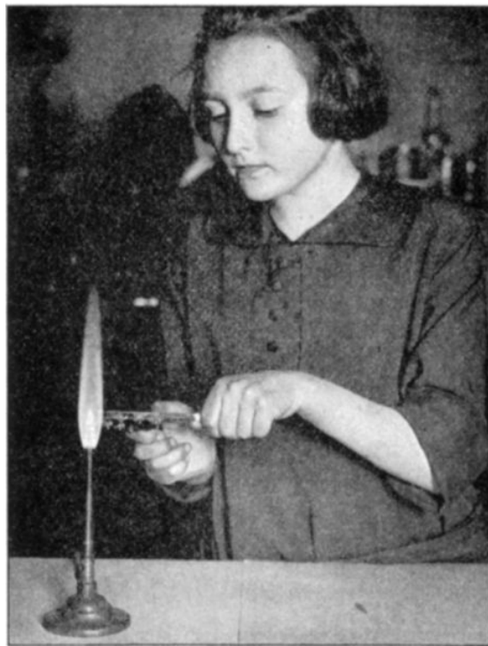
FIG. 57. Does the heat travel faster through the iron or through the glass?
