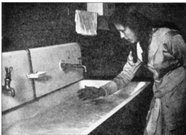
FIG. 102. When the wave reaches the end of the sink, it is reflected back. Sound waves are reflected in the same way.
