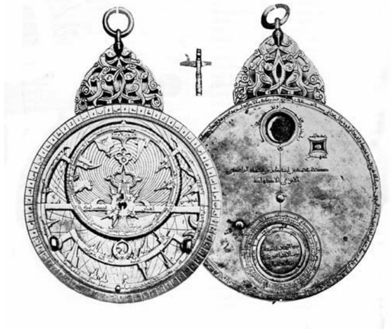
Figure 11.—GEARED ASTROLABE BY MUHAMMAD B. ABI BAKR OF ISFAHAN, A.D. 1221-1222. (Photo courtesy of Science Museum, London.)
