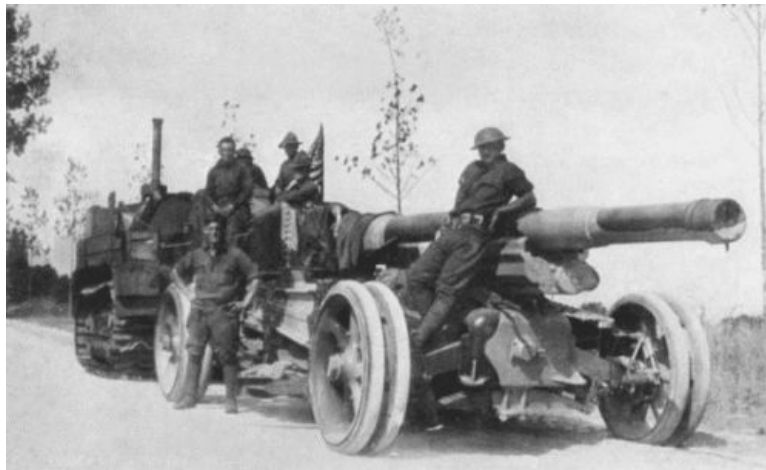
IN THE COURSE OF ITS PROGRESS TO THE VALLEY OF THE VESLE THIS 155 MM. GUN AND OTHERS OF ITS KIND WERE EDUCATING THE BOCHE TO RESPECT AMERICA. THE TRACTOR HAULS IT ALONG STEADILY AND SLOWLY, LIKE A STEAM ROLLER
