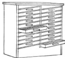
Fig. 39. Cabinet for Script Type, Borders, or other small characters which can be kept standing face up.
