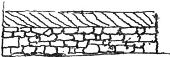
COB COURSE, OR SCAR, SHOWING DIAGONAL LAYERS.
