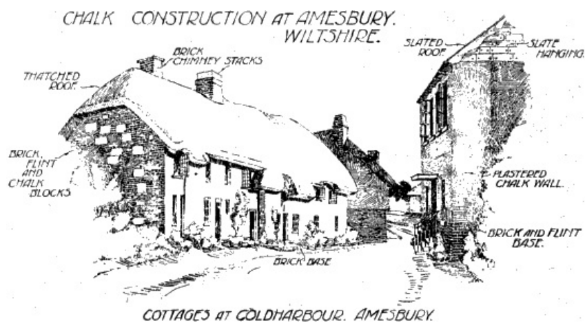
CHALK CONSTRUCTION AT AMESBURY, WILTS. (From a sketch by W. R. Jaggard, F.R.I.B.A., the copyright of the Department of Scientific and Industrial Research.)
