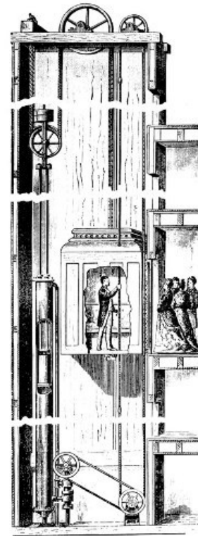
Figure 13.—Vertical cylinder, rope-gear hydraulic elevator with 2:1 gear ratio and rope control (about 1880).
