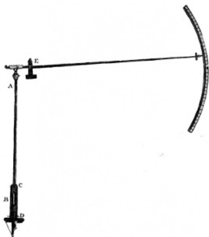
Figure 15.—"Steelyard barometer" as shown in Charles Hutton's Mathematical and Philosophical Dictionary (London, 1796, vol. 1, p. 188). Hutton makes no reference to the originator of this instrument; he attributes the "Diagonal" (or inclined) barometer to Samuel Morland.
