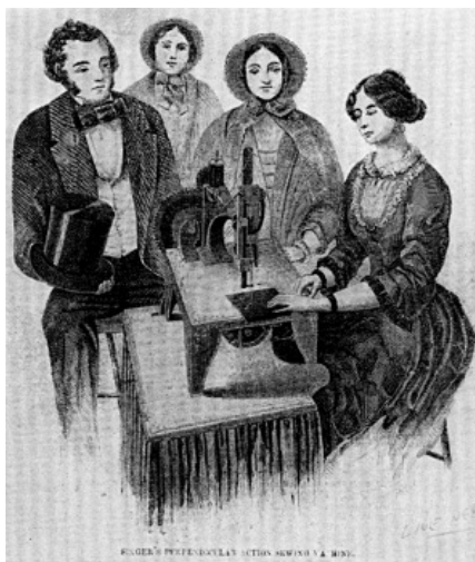
Figure 29.—SINGER'S PERPENDICULAR ACTION sewing machine, an engraving from Illustrated News , June 25, 1853, which states: "The sewing machine has, within the last two years acquired a wide celebrity, and established its character as one of the most efficient labor saving instruments ever introduced to
