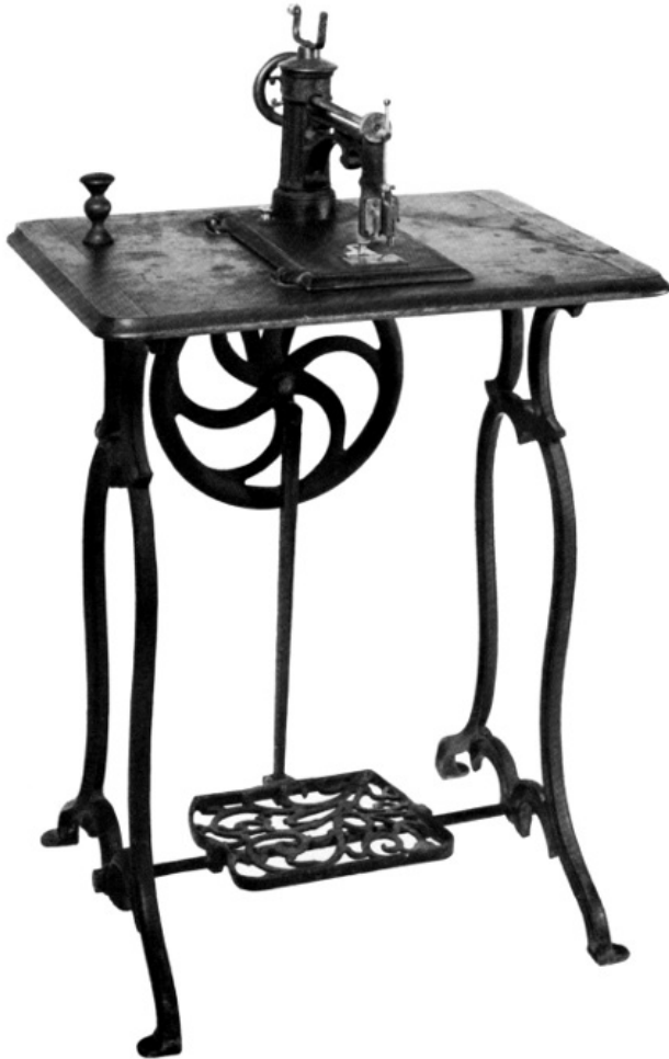
Figure 127.—WEST & WILLSON SEWING MACHINE of about 1859. The West & Willson machine, manufactured under the patent of H. B. West and H. F. Willson, enjoyed a very brief span of popularity. The patent covered the peculiar method of operating a spring-looper in combination with an eye-pointed needle to form a single chainstitch, but whether machines of this single-thread variety were manufactured is unknown. The machine illustrated here is a two-thread machine of basically the same description. It stitches from left to right and bears serial number 1544 and the inscription "West & Willson Co. patented June 29, 1858." (Smithsonian photo 49456-A.)
