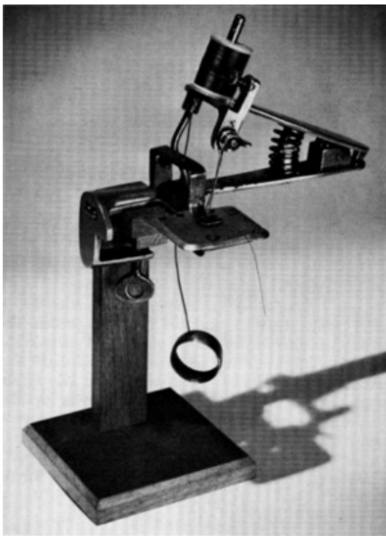
Figure 75.—BECKWITH SEWING MACHINE, 1871. Among the inventors whose patent claims were "to produce a cheap and effective sewing machine" was William G. Beckwith. His machine was first manufactured by Barlow & Son, and it realized considerable success in the few years of its production. The earliest model was operated like a pair of scissors or with a cord and ring as illustrated. Beckwith later added a hand crank. The machine was purchased in Crewe, Cheshire, England; it is stamped "Pat. April 18, 71 by Wm. G. Beckwith, Foreign Pats. Secured, Barlow & Son Manuf. N.Y., [serial number] 706." By 1874 the machines were marked "Beckwith S.M. Co." and two 1872 patent dates were added.
