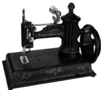
Figure 84.—GLOBE SEWING MACHINE. J. G. Folsom received two design patents in 1864, one on March 1 for a spool holder and one on May 17 for the basic style of the machine. Also in the same year, he was awarded a mechanical patent for an adjustment in the lower looper that would accommodate a change in needle size. Using these patents, he manufactured a single-thread, chainstitch machine, the Globe. Folsom also exhibited his machines at the Tenth Exhibition of the Massachusetts Charitable Mechanics Association in 1865. The Globe attracted particular attention and was awarded a silver medal.
