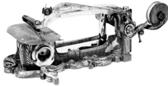
Figure 27.—WILSON'S four-motion-feed patent model, 1854, is not known to be in existence; this is a commercial machine of the period. The plate is stamped "A. B. Wilson, Patented Aug. 12, 1851, Watertown, Conn., No. 1...." (Smithsonian photo 45504.)
