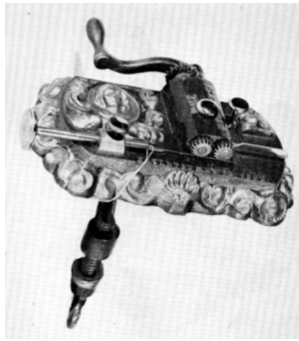
Figure 52.—THE FAIRY SEWING MACHINE sold for five dollars and was adequate for its advertised purpose, sewing or running very lightweight fabrics. The machine was marked with the Palmer patent, the date May 13, 1862, and the name “Mme. Demorest.”
