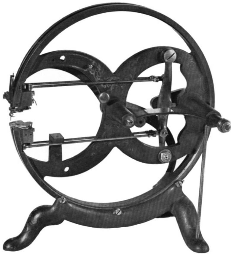
Figure 118.—SEWING MACHINE OF ABOUT 1856 with inscription “Howard & Davis Makers, Boston, Mass. Robinson & Roper Pat. Dec. 10, 1850, Aug. 15, 1854”; the drive wheel and the circular stitching plate of this machine are missing. (Smithsonian photo 48440-C.)
