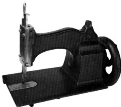
Figure 79.—CLARK'S Revolving-Looper double-thread sewing machine, 1860. This machine was manufactured by Lamson, Goodnow, & Yale of Windsor, Vermont. It was an attempt to improve on the combined ideas of the Grover and Baker machine, the Nettleton & Raymond machine, and the earlier single-thread Windsor machine. The improvements were made and patented by Edwin Clark on December 6, 1859. Widely advertised, the machines sold for $35 with a foot-power table. They could also be operated by hand. Over three thousand were manufactured and sold, and preparations were being made to continue manufacture of the earlier single-thread Windsor, originally made by the company's predecessor, Vermont Arms Co., when the Civil War broke out. A flood of arms orders arrived, and the sewing-machine manufacture was discontinued early in the summer of 1861. The sewing-machine equipment and business was sold to Grout & White of Massachusetts. (Smithsonian photo 48216.)
