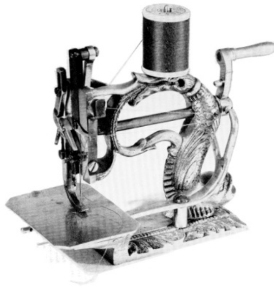
Figure 40.—A DOLPHIN sewing machine based on Clark’s patent of 1858. This design was first used by T. J. W. Robertson in 1855, but in his patent issued on May 22 of that year no claim was made for the machine design, only for the chainstitch mechanism. The same style was used by D. W. Clark in several of his chainstitch patents, but he also made no claim for the design, stating that the machine “may be made in any desired ornamental form.” The dolphin-style machines are all chainstitch models of solid brass, originally gilt. Although only about five inches long, they are full-size machines using a full-size needle. (Smithsonian photo 45505.)
