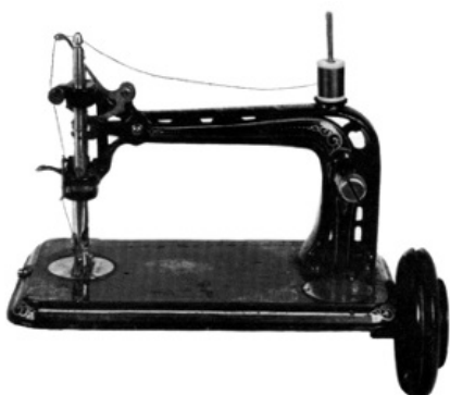
Figure 68.—AMERICAN BUTTONHOLE, Overseaming & Sewing Machine of about 1870. Using serial numbers, these machines can be dated approximately as follows: 1-7792, 1869; 7793-22366, 1870; 22367-42488, 1871; 42489-61419, 1872; 61420-75602, 1873; 75603-89132, 1874; 89133-103539, 1875; and 103540-121477, 1876. Figures are not available for the years from 1877 to 1886. (Smithsonian photo 46953-E.)
