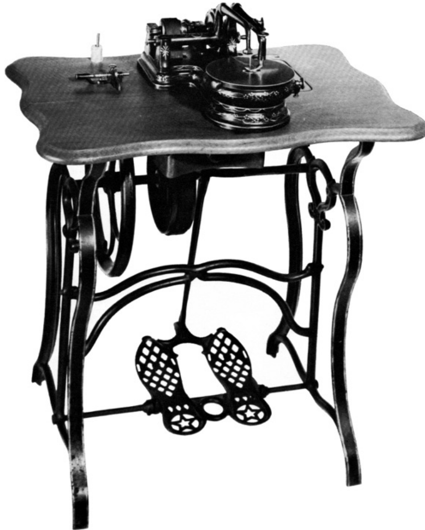
Figure 83.—FLORENCE SEWING MACHINE. The Florence machine was based on the patents of Leander W. Langdon, whose first patent was obtained in 1855. Langdon sewing machines were manufactured by the inventor for a few years. It was his patent of March 20, 1860, that was the immediate forerunner of the Florence machine, whose name was derived from the city of manufacture, Florence, Massachusetts. The Howe royalty records of 1860 listed the Florence Sewing Machine Co. as one that took out a license that year. Langdon's patent of July 14, 1863, was incorporated into the machines manufactured after that date; however, the date is always incorrectly stamped "July 18, 1863." In 1865, the machine won a silver medal at the Tenth Exhibition of the Massachusetts Charitable Mechanics Association.
