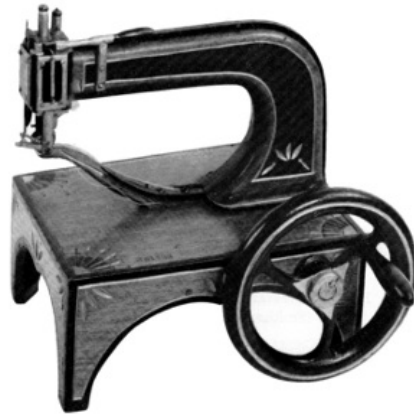
Figure 55.—BLAKE'S LEATHER-STITCHING MACHINE patent model of July 6, 1858; the inventor claimed the arrangement of the mechanism used and an auxiliary arm capable of entering the shoe, which enabled the outer sole to be stitched both to the inner sole and to the upper part of the shoe. (Smithsonian photo 50361.)
