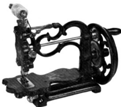
Figure 102.—IMPROVED COMMON SENSE sewing machine of about 1870. This machine is so very similar to the New England machines in its feed, threading, looping mechanism, and in its general design, that it is sometimes mistaken for the earlier New England machines (see figs. 112 and 113).
