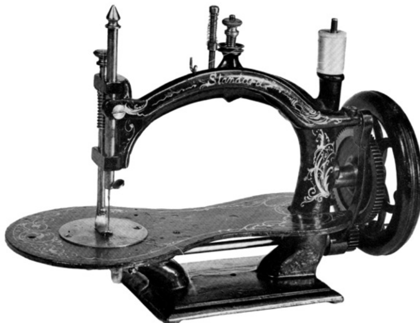
Figure 123.—STANDARD SEWING MACHINE of about 1870. This chainstitch machine is believed to have been made by the company that later became the Standard Shuttle Sewing Machine Company, when they began manufacturing lockstitch machines about 1874. This machine is marked with the name, "Standard," and with the dates "Patented July 14, 1870, Patented Jan. 22, 1856, Dec. 9, 1856, Dec. 12, 1865." The dates refer to the reissue and extended reissue of the Bachelder and the A. B. Wilson patents. The number of chainstitch machines of this type that were manufactured is not known. (Smithsonian photo 45506-C.)
