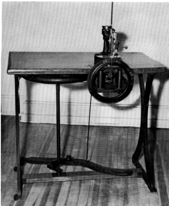
Figure 72.—A. BARTHOLF SEWING MACHINE, 1853. Abraham Bartholf of New York began manufacturing Blodgett & Lerow machines (see fig. 20) about 1850; the style and mechanics of these machines, however, were primarily those of the Blodgett & Lerow patent as manufactured by O. C. Phelps and Goddard, Rice & Co. For this reason they are considered Blodgett & Lerow—not Bartholf—machines.
