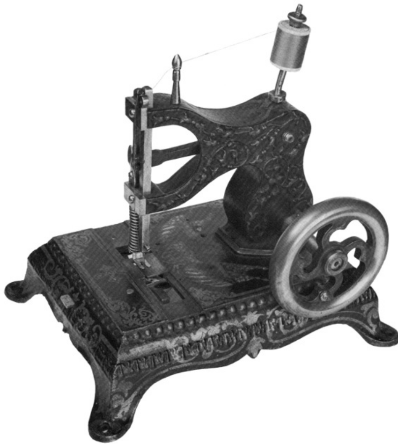
Figure 110.—NE PLUS ULTRA of about 1867. Another of the interesting hand-turned chainstitch machines of the late 1850s and 1860s was patented by O.L. Reynolds. The baster plates and the handle on the wheel are missing on this machine, but an interesting shield and draped-flag pattern is painted on the base.
