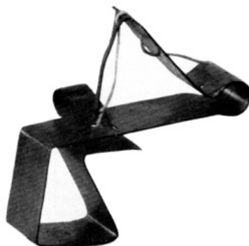
Figure 48.—HEYER'S POCKET SEWING MACHINE patent model, November 17, 1863. This patent model is one piece, and measures about
