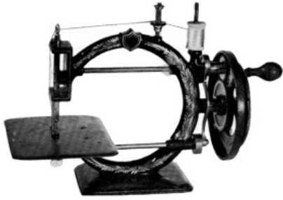
Figure 73.—BARTLETT SEWING MACHINE, 1867. The Bartlett machine was first manufactured in 1866 under the January 31, 1865, and October 10, 1865, patents of Joseph W. Bartlett. The machines were made by Goodspeed & Wyman for the Bartlett Co. and were so marked. The inventor received another patent on April 7, 1868, and later machines carry this third date also. Although the first few hundred machines did not bear the dates of patents held by the "Combination," before the end of the first year of production Bartlett was paying royalties. He continued to manufacture sewing machines until the early seventies when he converted to the manufacturing of street lamps.
