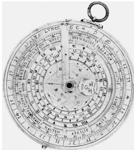
FIGURE 3.—Lunar dial, Germany, 1604. Concentric scales mark hours of the day, days, months, and special astrological numbers. In conjunction with other dials, it enables the user to determine the phases of the moon. (NMHT 30121; SI photo P-63426.)
