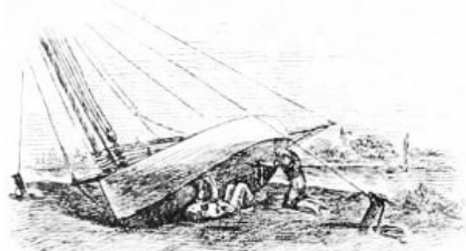
METHOD OF SCRAPING BOTTOM.
