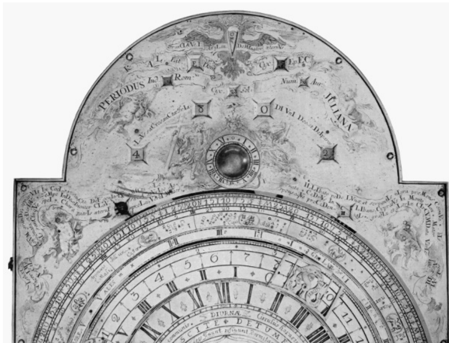
Figure 16. —DETAIL OF FRONTISPIECE of the Borghesi clock, showing the apertures for calendar indicators and the details of the engraving.
