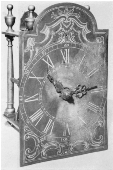
Figure 26.—DIAL PLATE of a brass lantern clock made by Bertolla, found in his workshop after his death. (Courtesy of Museo Nazionale della Scienza e della Tecnica, Milan.)
