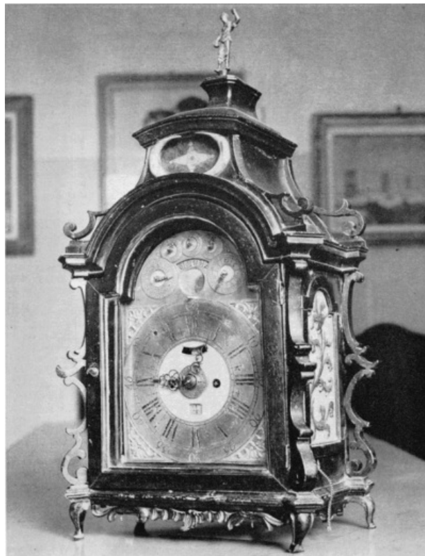
Figure 29.—TABLE CLOCK BY BERTOLLA in the collection of Doctor Vittorio dal Lago of Bergamo. The dial indicates the days of the week and of the month, the names of the months and lunar phases. The clock strikes the hours and quarters and repeats. (Courtesy of Sig. Luigi Pippa of Milan.)
