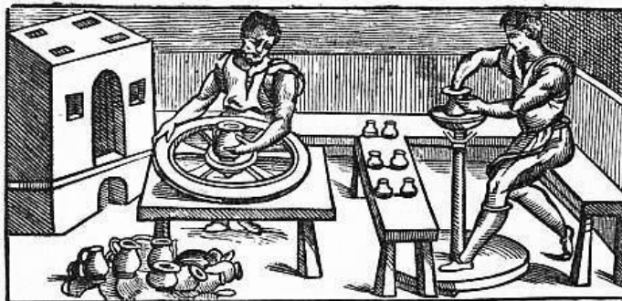
FIG. 5.—Two forms of Italian potter's wheels, about 1540.
