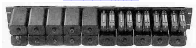
Fig. 367. Strip of Kellogg Line and Cut-Off Relays View full size illustration.
