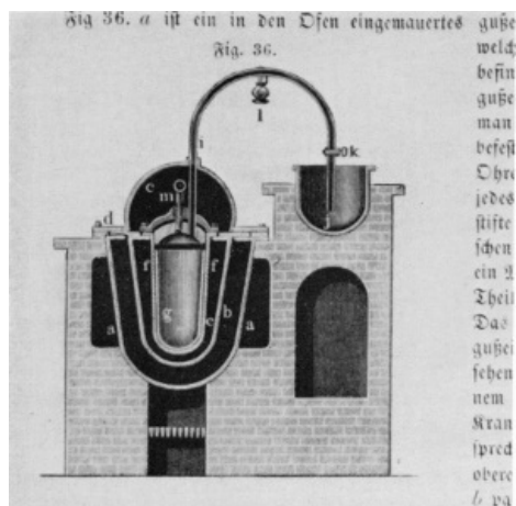
Figure 4.—APPARATUS FOR CONVERTING WHITE PHOSPHORUS into the red allotropic form, 1851. Redistilled phosphorus is heated in the glass or porcelain vessel (g) which is surrounded by a sandbath (e) and a metal bath (b). Vessel (j) is filled with mercury and water; together with valve (k), it serves as a safety device. The alcohol lamp (l) keeps the tube warm against clogging by solidified vapors. Because of hydrogen phosphides, the operation, carried out at 260° C., had to be watched very carefully. (According to Arthur Albright, 1851; reproduced from HUGO FLECK, Die Fabrikation chemischer Produkte ... , page 112.)
