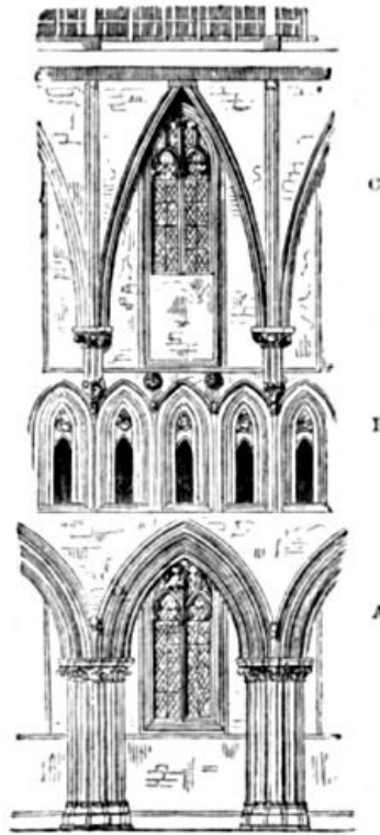
FIG. 5.—NAVE OF WELLS CATHEDRAL. (1206 TO 1242.) A. Nave Arcade. B. Triforium. C. Clerestory.
