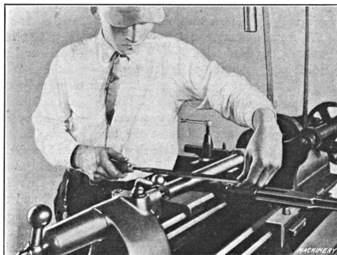
Fig. 11. Filing Work after Finishing Cut is taken
