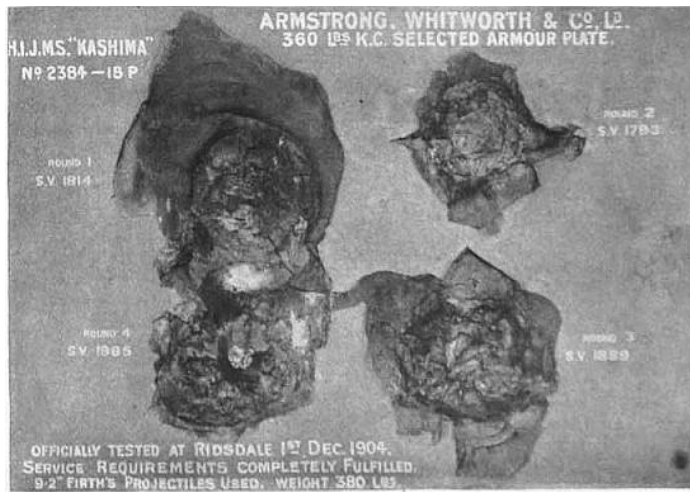
FIG. 4.—KRUPP-CEMENTED PLATE, 9 INCHES THICK, AFTER ATTACK. (ARMSTRONG, WHITWORTH & CO.)
