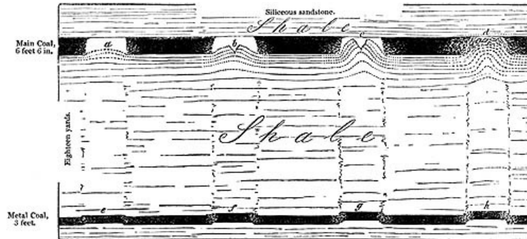
Section of carboniferous strata, at Wallsend, Newcastle, showing "Creeps." (J. Buddle, Esq.) Horizontal length of section 174 feet. The upper seam, or main coal, here worked out, was 630 feet below the surface.
