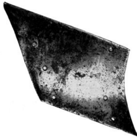
Figure 5.—MOLDBOARD OF 1847 JOHN DEERE PLOW, showing how the diamond shape of the original design has been slightly modified. (Deere & Company photo 57192-D.)
