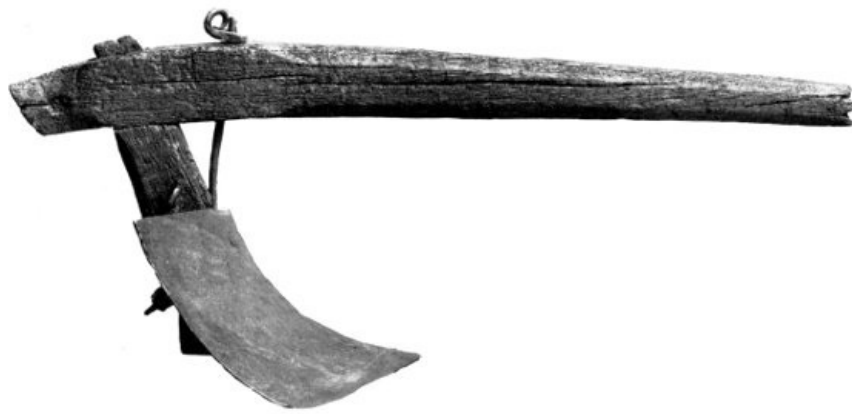
Figure 7.—JOHN DEERE'S 1838 PLOW, RIGHT SIDE, showing large iron staple used to fasten end of right handle to the standard. Note remains of wooden pin near rear end of plow beam. (Cat. no. F1111; Smithsonian photo 42639-A.)
