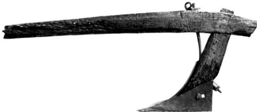
Figure 9.—JOHN DEERE'S 1838 PLOW, LEFT SIDE, showing details of construction and relationship of landside to moldboard. (Cat. no. F1111; Smithsonian photo 42639.)
