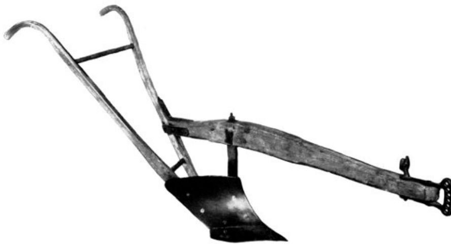
Figure 6.—THE SHAPE OF THE MOLDBOARD continued to evolve, as illustrated by this 1855 John Deere plow. (Deere & Company photo 57192-A.)
