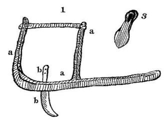
No. 1 is a plough drawn by a horse. b, b, is a strong thick-backed knife, placed in the middle of the plough, and serving to cut straight lines through the grassy turf, which in the course of five or six years has accumulated on the soil.
