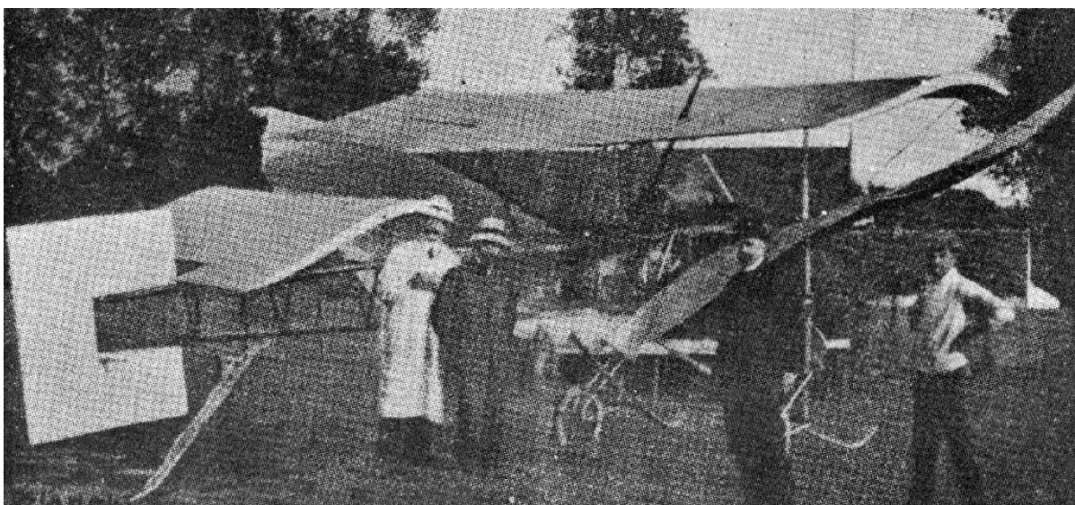
DE LA HAULT II. (1910-11). The ornithopter principle applied to a monoplane. No success met with.
