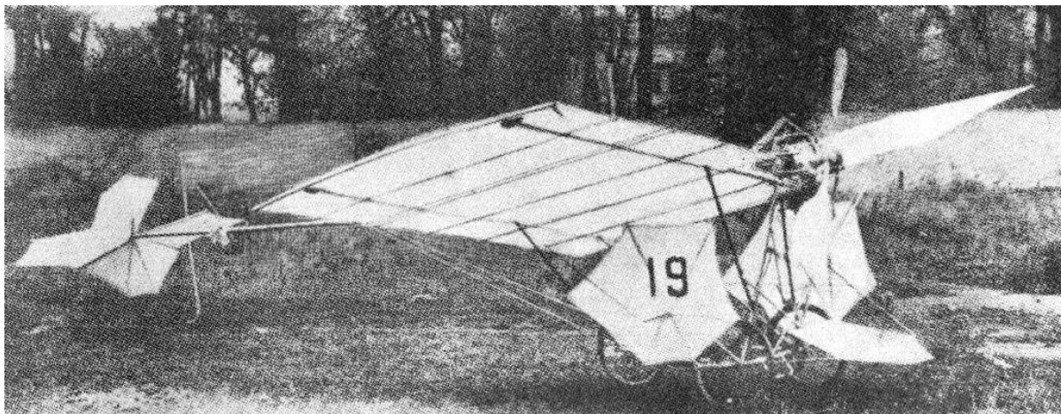
SANTOS-DUMONT XIX . This little machine, surface only 9 m 2 , made an extraordinary sensation in France in 1909. It flew at the then incredible speed of 65 m.p.h. (100 k.p.h.) Santos-Dumont presented all rights to the world soon afterwards, and a large number were built before it was realised that only an extremely light weight pilot could fly in one. Few of the copies ever left the ground.
