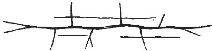
Fig. 18.—Ground-plan of Large Main Fault and Minor Displacement Fissures.
