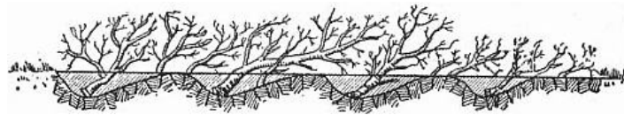
From Mil. Engineering: Field Defences , by permission of the Controller H.M. Stationery Office. FIG. 93.—Abatis.
