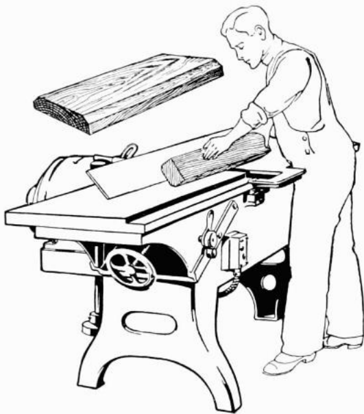
Fig. 41. Cutting bevels on jointer
