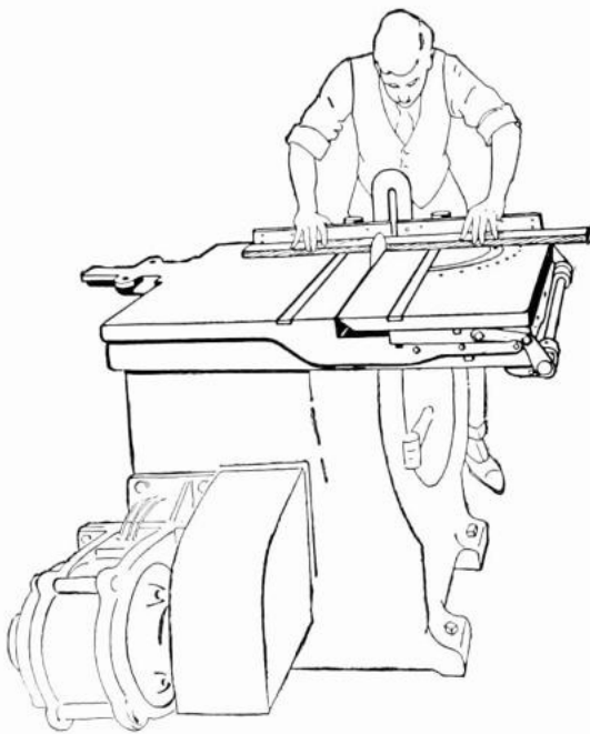
Fig. 37. Cutting with special fence
