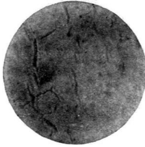
15. Test No. 6 on 1906 Fence. Surface Checking Only
