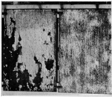
Plate Showing Effect of Chemically Active Pigments on Oil after One Year's Wear
