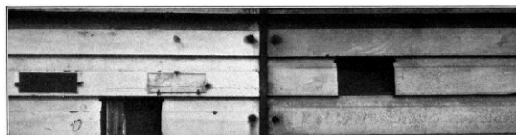
Whiteness of Sublimed White Lead Darkness of Corroded White Lead On Pittsburg Test Fence
