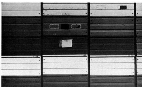
Panels on Atlantic City Fence Two Lower Sets of Panels are Painted with Combination Pigment Paints. Excellent Results shown
