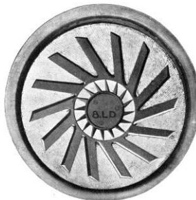
View showing careful Dressing of Bull Stone Mill from Grinder
