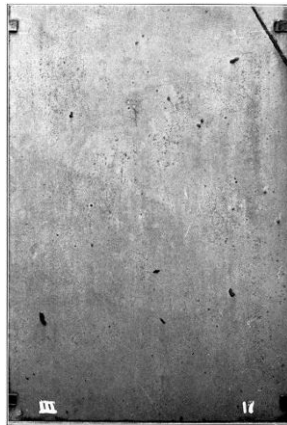
Corrosion Pits on Graphite Panel
