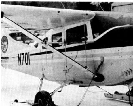
Figure 13.—Directional yagi antennas fastened to the wing struts of the aircraft were necessary to "home in" on the wolves. (Photo courtesy of U.S. Bureau of Sport Fisheries and Wildlife.)
