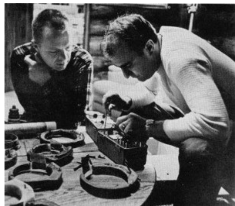
Figure 12.—Each radio collar had a different frequency tuned to special receivers, which allowed each wolf to be identified. (Photo courtesy of D. L. Breneman.)
