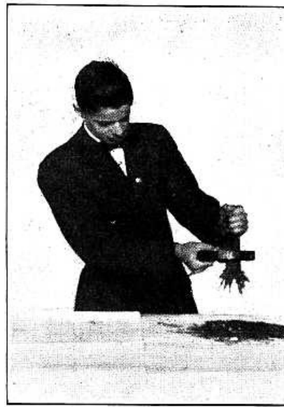
FIG. 23—A BAR OF SOFT IRON WITH A CURRENT FLOWING AROUND IT BECOMES A MAGNET
