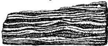
Fragment of gneiss; section made at right angles to the planes of foliation.
