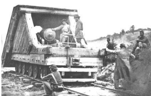
Curious Federal soldiers inspect a Confederate armored gun, the earliest rail artillery on record. This "land ram", designed by Lt. John M. Brooke of the Confederate Navy, was first used at Savage Station, Virginia, in 1862.
