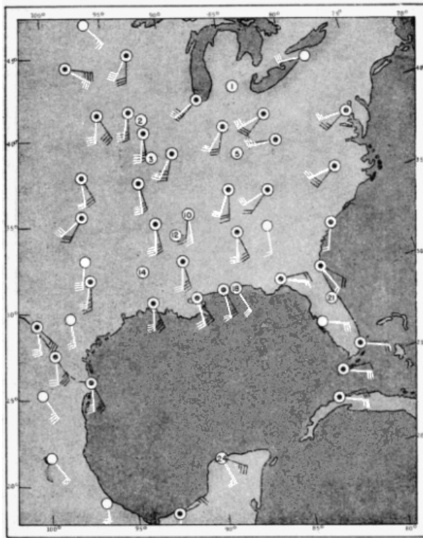
FIG. 45. Winds aloft at 10:00 P. M. on April 24 (CST). Winds at 2,000 feet above mean sea level are shown in black; those at 4,000 feet, in white. Velocities are indicated by standard Beaufort Scale of Wind Force. The numbers in circles refer to the stations shown in Figure 44 .
