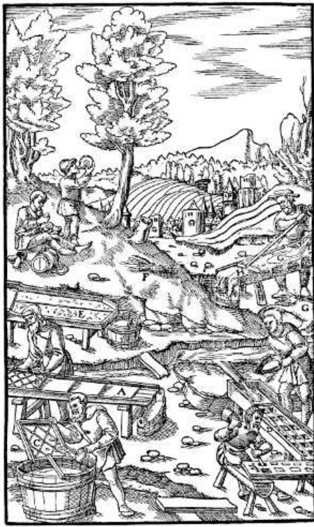
A—SLUCE COVERED WITH CANVAS. B—ITS HEAD FULL OF POCKETS AND GROOVES. C—HEAD REMOVED AND WASHED IN A TUB. D—SLUCE WHICH HAS SQUARE POCKETS. E—SLUCE TO WHOSE PLANKS SMALL SHAVINGS CLING. F—BROOM. G—SKINS OF OXEN. H—WOODEN SCRUBBER. [Pg 329]
