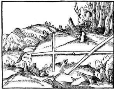
A—PRINCIPAL VEIN. B—TRANSVERSE VEIN. C—VEIN CUTTING PRINCIPAL ONE OBLIQUELY. [Pg 64]
