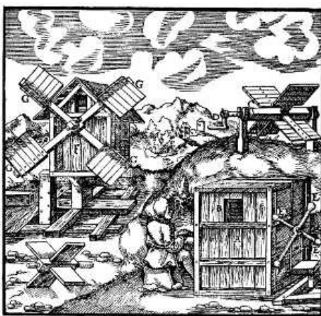
A—BOX-SHAPED CASING PLACED ON THE GROUND. B—ITS BLOW-HOLE. C—ITS AXLE WITH FANS. D—CRANK OF THE AXLE. E—
