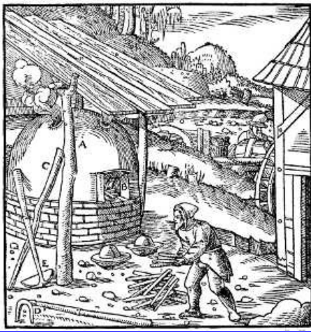
A—FURNACE. B—ITS MOUTH. C—POKER. D—RAKE WITH TWO TEETH. E—HOE. [Pg 349]
