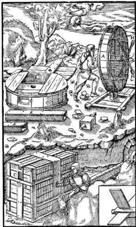
A—DRUM. B—BOX-SHAPED CASING. C— BLOW-HOLE. D—SECOND HOLE. E— CONDUIT. F—AXLE. G—LEVER OF AXLE. H —RODS. [Pg 204]
