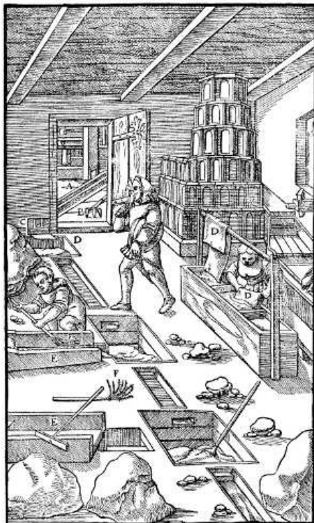
A—LAUNDER FROM THE SCREEN OF THE MORTAR-BOX. B—THREE-TOOTHED RAKE. C—SMALL SETTling-PIT. D—CANVAS. E—STRAKES. F—BROOMS. [Pg 317]
