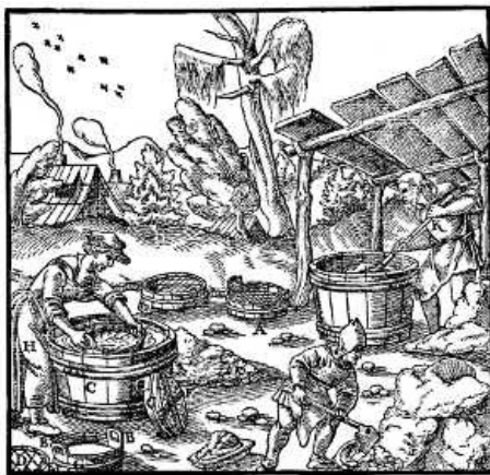
A—SIEVE. B—ITS HANDLES. C—TUB. D—BOTTOM OF SIEVE MADE OF IRON WIRES. E—HOOP. F—RODS. G—HOOPS. H—WOMAN SHAKING THE SIEVE. I—BOY SUPPLYING IT WITH MATERIAL WHICH REQUIRES WASHING. K—MAN WITH SHOVEL REMOVING FROM THE TUB THE MATERIAL WHICH HAS PASSED THROUGH THE SIEVE. [Pg 292]
