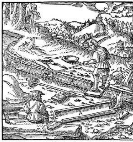
A—TROUGH. B—ITS OPEN END. C—END THAT MAY BE CLOSED. D—STREAM. E—HOE. F—END-BOARD. G—BAG. [Pg 335]
