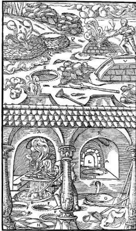
A—FURNACE OF THE CARNI. B—LOW WALL. C—WOOD. D—ORE DRIPPING LEAD. E—LARGE CRUCIBLE. F—MOULDS. G—LADLE. H—SLABS OF LEAD. I—RECTANGULAR HOLE AT THE BACK OF THE FURNACE. K—SAXON FURNACE. L—OPENING IN THE BACK OF THE FURNACE. M—WOOD. N—UPPER CRUCIBLE. O—DIPPING-POT. P—WESTPHALIAN METHOD OF MELTING. Q—HEAPS OF CHARCOAL. R—STRAW. S—WIDE SLABS. T—CRUCIBLES. V—POLISH HEARTH. [Pg 393]
