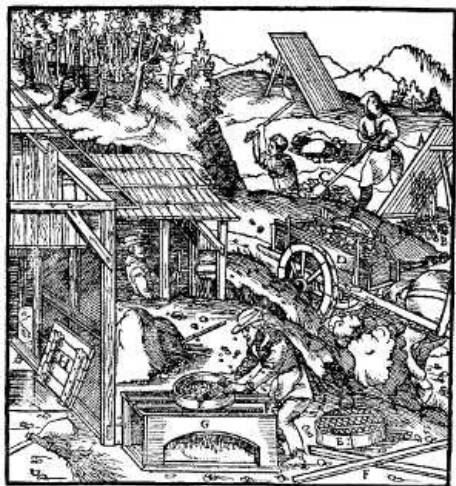
A—SCREEN. B—POLES. C—SHOVEL. D—TWO-WHEELED CART. E—HAND-SIEVE. F—NARROW BOARDS. G—BOX. H—COVERED PIT. [Pg 375]
