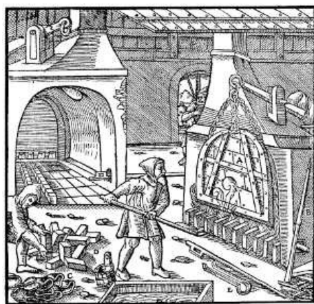
A—THE DOOR LET DOWN. B—BAR. C— EXHAUSTED LIQUATION CAKES. D—BRICKS. E—TONGS. [Pg 527]
