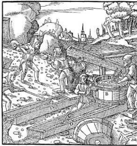
A—SIEVE. B—TUB. C—WATER FLOWING OUT OF THE BOTTOM OF IT. D—STRAKE. E—THREE-TOOTHED RAKE. F—WOODEN SCRUBBER. [Pg 342]
