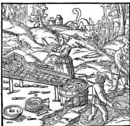
A—PLANK. B—SIDE-BOARDS. C—IRON WIRE. D—HANDLES. [Pg 324]
