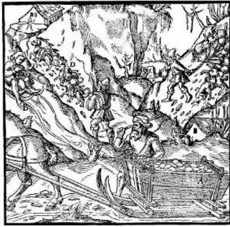
A—SLEDGE WITH BOX PLACED ON IT. B—SLEDGE WITH SACKS PLACED ON IT. C—STICK. D—DOGS WITH PACK-SADDLES. E—PIGSKIN SACKS TIED TO A ROPE. [Pg 168]
