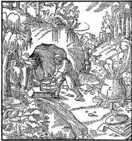
A—BITUMINOUS SPRING. B—BUCKET. C— POT. D—LID. [Pg 583]
