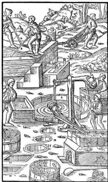
A—TANKS. B—STIRRING POLES. C—PLUG. D—TROUGH. E—RESERVOIR. F— LAUNDER. G—LEAD CALDRON. H—WOODEN TUBS SUNK INTO THE EARTH. I—VATS IN WHICH TWIGS ARE FIXED. [Pg 567]
