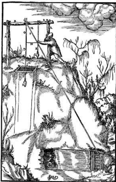
A—UPRIGHT FORKED POSTS. B—POLE OVER THE POSTS. C—SHAFT. D—FIRST CORD. E—WEIGHT OF FIRST CORD. F—SECOND CORD. G—SAME FIXED GROUND. H—HEAD OF FIRST CORD. I—MOUTH OF TUNNEL. K—THIRD CORD. L—WEIGHT OF THIRD CORD. M—FIRST SIDE MINOR TRIANGLE. N—SECOND SIDE MINOR TRIANGLE. O—THIRD SIDE MINOR TRIANGLE. P—THE MINOR TRIANGLE. [Pg 131]
