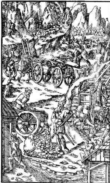
A—HORSES WITH PACK-SADDLES. B—LONG BOX PLACED ON THE SLOPE OF THE CLIFF. C—CLEATS THEREOF. D—WHEELBARROW. E—TWO-WHEELED CART. F—TRUNKS OF TREES. G—WAGON. H—ORE BEING UNLOADED FROM THE WAGON. I—BARS. K—MASTER OF THE WORKS MARKING THE NUMBER OF CARTS ON A STICK. L—BOXES INTO WHICH ARE THROWN THE ORE WHICH HAS TO BE DIVIDED. [Pg 170]
