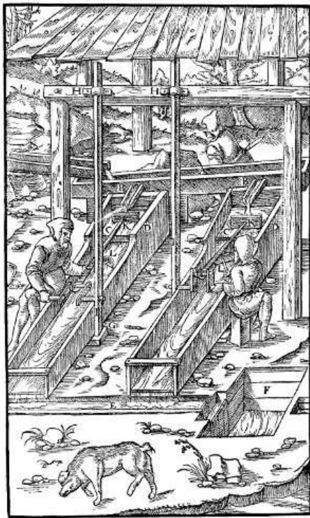
A—UPPER CROSS LAUNDER. B—SMALL LAUNDERS. C—HEADS OF STRAKES. D—STRAKES. E—LOWER TRANSVERSE LAUNDER. F—SETTLING PIT. G—SOCKET IN THE SILL. H—HALVED IRON RINGS FIXED TO BEAM. I—POLE. K—ITS LITTLE SCRUBBER. L—SECOND SMALL SCRUBBER. [Pg 305]
