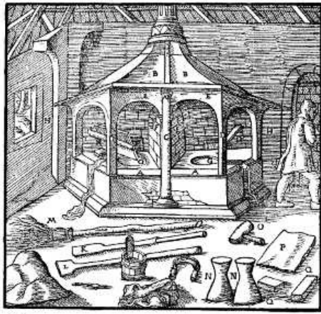
A—HEARTH OF THE FURNACE. B—CHIMNEY. C—COMMON PILLAR. D—OTHER PILLARS. THE PARTITION WALL IS BEHIND THE COMMON PILLAR AND NOT TO BE SEEN. E—ARCHES. F—LITTLE WALLS WHICH PROTECT THE PARTITION WALL FROM INJURY BY THE FIRE. G—CRUCIBLES. H—SECOND LONG WALL. I—DOOR. K—SPATULA. L—THE OTHER SPATULA. M—THE BROOM IN WHICH IS INSERTED A STICK. N—PESTLES. O—WOODEN MALLET. P—PLATE. Q—STONES. R—IRON ROD. [Pg 532]
