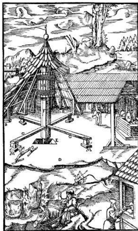
A—UPRIGHT BEAMS. B—SILLS LAID FLAT UPON THE GROUND. C—POSTS. D—AREA. E—SILL SET AT THE BOTTOM OF THE HOLE. F—AXLE. G—DOUBLE CROSS-BEAMS. H—DRUM. I—WINDING-ROPE. K—BUCKET. L—SMALL PIECES OF WOOD HANGING FROM DOUBLE CROSS-BEAMS. M—SHORT WOODEN BLOCK. N—CHAIN. O—POLE BAR. P—GRAPPLING HOOK. (Some members mentioned in the text are not shown). [Pg 165]
