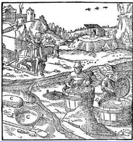
A—BASKET. B—ITS HANDLES. C—DISH. D—ITS BACK PART. E—ITS FRONT PART. F—HANDLES OF SAME. [Pg 293]
