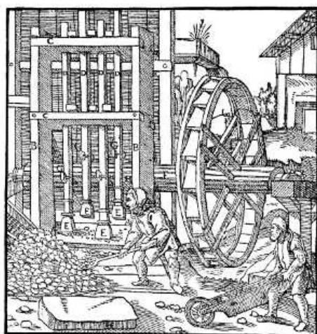
A—MORTAR. B—UPRIGHT POSTS. C—CROSS-BEAMS. D—STAMPS. E—THEIR HEADS. F—AXLE (CAM-SHAFT). G—TOOTH OF THE STAMP (TAPPET). H—TEETH OF AXLE (CAMS). [Pg 284]
