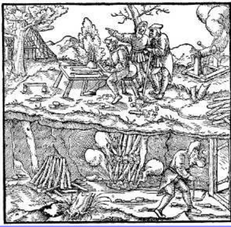
A—KINDLED LOGS. B—STICKS SHAVED DOWN FAN-SHAPED. C—TUNNEL. [Pg 120]
