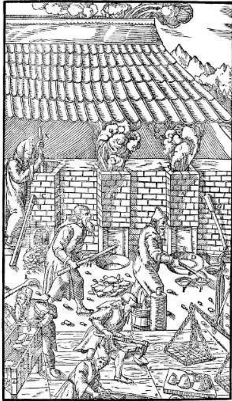
A, B, C—THREE FURNACES. AT THE FIRST STANDS THE SMELTER, WHO WITH A LADLE POURS THE ALLOY OUT OF THE FOREHEARTH INTO THE MOULDS. D—FOREHEARTH. E—LADLE. F—MOULDS. G—ROUND WOODEN RAMMER. H—TAPPING-BAR. AT THE SECOND FURNACE STANDS THE SMELTER, WHO OPENS THE TAP-HOLE WITH HIS TAPPING-BAR. THE ASSISTANT, STANDING ON STEPS PLACED AGAINST THE THIRD FURNACE WHICH HAS BEEN BROKEN OPEN, CHIPS OFF THE ACCRETIONS. I—STEPS. K—SPATULA. L—THE OTHER HOOKED BAR. M—MINE CAPTAIN CARRYING A CAKE, IN WHICH HE HAS STUCK THE PICK, TO THE SCALES TO BE WEIGHED. N—ANOTHER MINE CAPTAIN OPENS A CHEST IN WHICH HIS THINGS ARE KEPT. [Pg 383]
