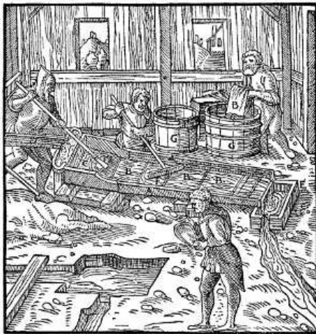
A—BEAMS. B—CANVAS. C—HEAD OF STRAKE. D—SMALL LAUNDER. E—SETTLING PIT OR TANK. F—WOODEN SCRUBBER. G—TUBS. [Pg 308]
