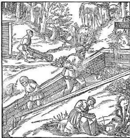
A—LAUNDER. B—INTERLACING FIR TWIGS. C—LOGS; THREE ON ONE SIDE, FOR THE FOURTH CANNOT BE SEEN BECAUSE THE DITCH IS SO FULL WITH MATERIAL NOW BEING WASHED. D—LOGS AT THE HEAD OF THE DITCH. E—BARROW. F—SEVEN-PRONGED FORK. G—HOE. [Pg 340]
