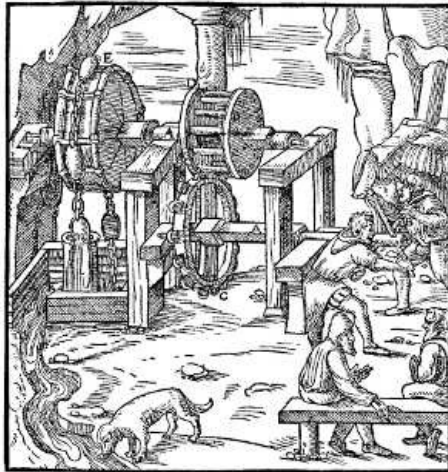
A—AXLES. B—LEVERS. C—TOOTHED DRUM. D—DRUM MADE OF RUNDLES. E— DRUM IN WHICH IRON CLAMPS ARE FIXED. [Pg 195]
