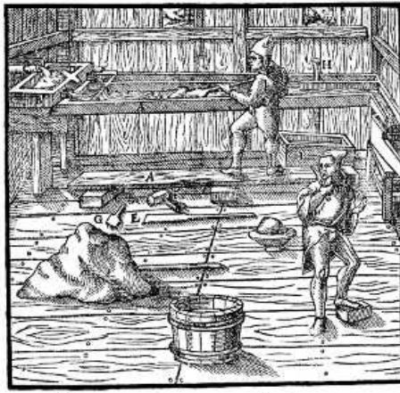
A—STRAKES. B—TANK. C—LAUNDER. D—PLUG. E—WOODEN SHOVEL. F—WOODEN Mallet. G—WOODEN SHOVEL WITH SHORT HANDLE. H—THE PLUG IN THE STRAKE. I—TANK PLACED UNDER THE PLUG. [Pg 341]
