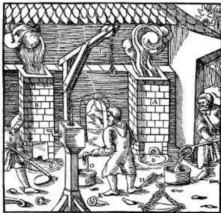
A—FURNACE IN WHICH "SLAGS" ARE RE-SMELTED. B—FURNACE IN WHICH COPPER IS ALLOYED WITH LEAD. C—DOOR. D—FOREHEARTHES ON THE GROUND. E—COPPER MOULDS. F—RABBLE. G—HOOK. H—CLEFT STICK. I—ARM OF THE CRANE. K—THE HOOK OF ITS CHAIN. [Pg 508]
