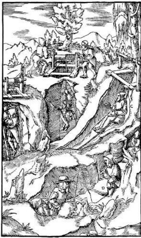
A—DESCENDING INTO THE SHAFT BY LADDERS. B—BY SITTING ON A STICK. C—BY SITTING ON THE DIRT. D—DESCENDING BY STEPS CUT IN THE ROCK. [Pg 213]
