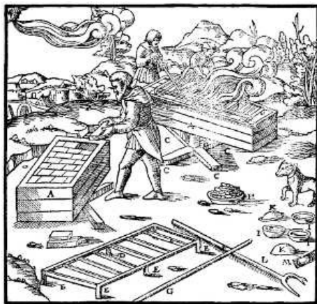
A—BOX. B—PIVOT. C—TRANSVERSE WOOD BEAMS. D—GRATE. E—ITS FEET. F—BURNING WOOD. G—STICK. H—PANS IN WHICH THE BISMUTH IS MELTED. I—PANS FOR MOULDS. K—CAKES. L—FORK. M—BRUSH. [Pg 437]
