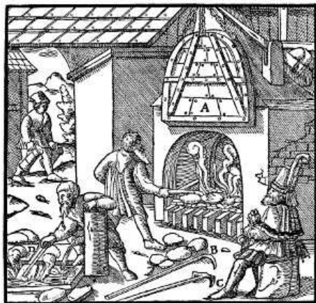
A—THE DOOR RAISED. B—HOOKED BAR. C— —TWO-PRONGED RAKE. D—TONGS. E— TANK. [Pg 528]
