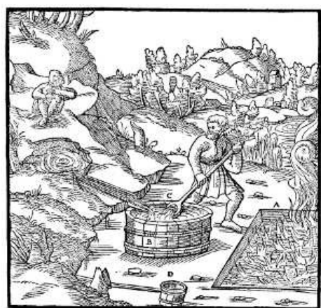
A—TRENCH. B—VAT INTO WHICH THE SALT WATER FLOWS. C—LADLE. D—SMALL BUCKET WITH POLE FASTENED INTO IT. [Pg 556]
