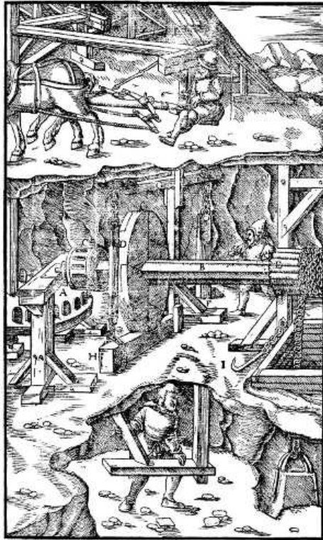
A—TOOTHED DRUM WHICH IS ON THE UPRIGHT AXLE. B—HORIZONTAL AXLE. C—DRUM WHICH IS MADE OF RUNDLES. D—WHEEL NEAR IT. E—DRUM MADE OF HUBS. F—BRAKE. G—OSCILLATING BEAM. H—SHORT BEAM. I—HOOK. [Pg 167]
