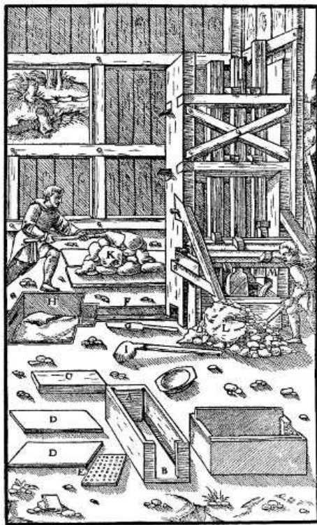
A—MORTAR. B—OPEN END OF MORTAR. C—SLAB OF ROCK. D—IRON SOLE PLATES. E—SCREEN. F—LAUNDER. G—WOODEN SHOVEL. H—SETTLING PIT. I—IRON SHOVEL. K—HEAP OF MATERIAL WHICH HAS SETTLED. L—ORE WHICH REQUIRES CRUSHING. M—SMALL LAUNDER. [Pg 313]
