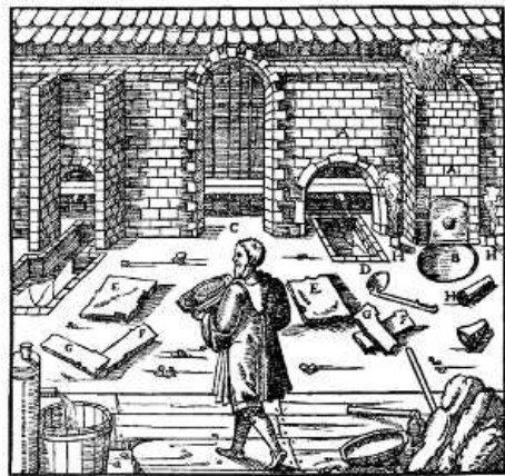
A—FURNACES. B—FOREHEARTH. C—DOOR. D—WATER TANK. E—STONE WHICH COVERS IT. F—MATERIAL OF THE VENT WALLS. G—STONE WHICH COVERS IT. H—PIPE EXHALING THE VAPOUR. [Pg 358]
