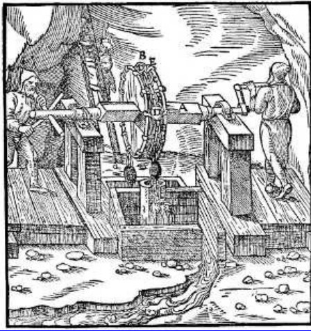
A—AXLE. B—DRUM. C—DRAWING-CHAIN. D—BALLS. E—CLAMPS. [Pg 194]
