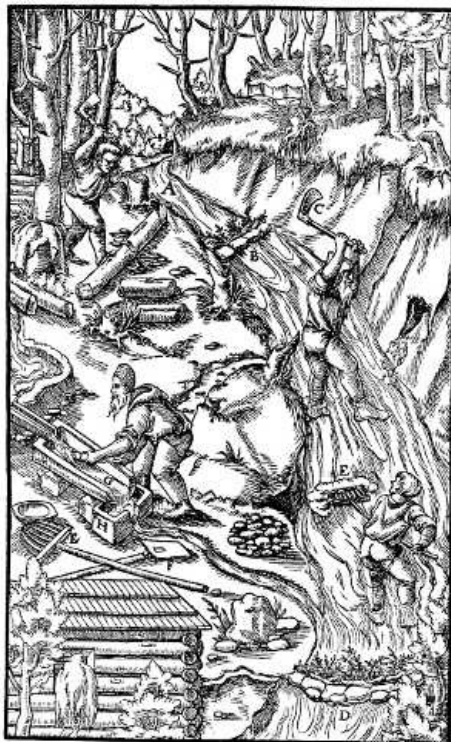
A—STREAM. B—DITCH. C—MATTOCK. D—PIECES OF TURF. E—SEVEN-PRONGED FORK. F—IRON SHOVEL. G—TROUGH. H—ANOTHER TROUGH BELOW IT. I—SMALL WOODEN TROWEL. [Pg 337]
