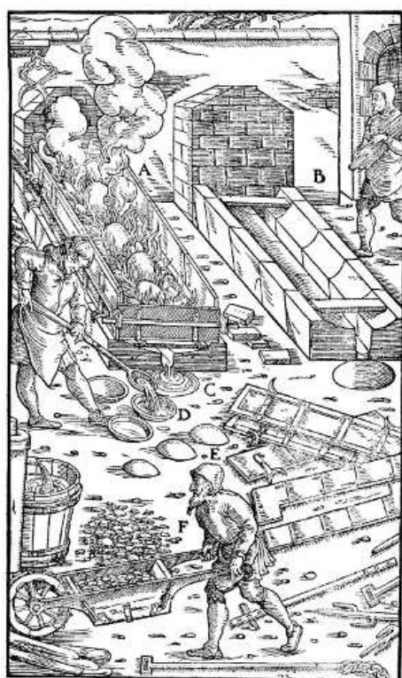
A—FURNACE IN WHICH THE OPERATION OF LIQUATION IS BEING PERFORMED. B—
