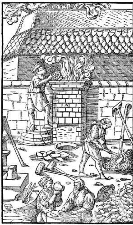
A—FURNACE. B—STAIRS. C—ORE. D—CHARCOAL. [Pg 424]
