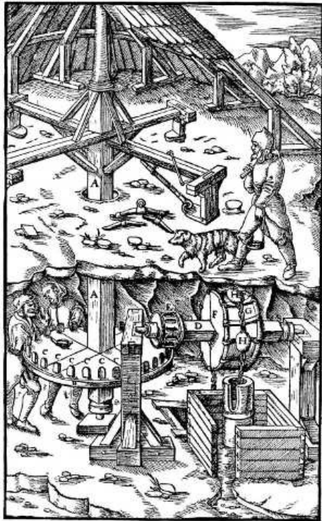
A—UPRIGHT AXLE. B—TOOTHED WHEEL. C—TEETH. D—HORIZONTAL AXLE. E—DRUM WHICH IS MADE OF RUNDLES. F—SECOND DRUM. G—DRAWING-CHAIN. H—THE BALLS. [Pg 193]
