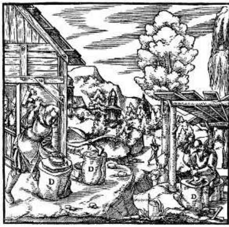
A—MASSES OF METAL. B—HAMMER. C—CHISEL. D—TREE STUMPS. E—IRON TOOL SIMILAR TO A PAIR OF SHEARS. [Pg 269]
