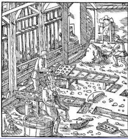
A—STAMPS. B—MORTAR. C—PLATES FULL OF HOLES. D—TRANSVERSE LAUNDER. E—PLANKS FULL OF CUP-LIKE DEPRESSIONS. F—SPOUT. G—BOWL INTO WHICH THE CONCENTRATES FALL. H—CANVAS STRAKE. I—BOWLS SHAPED LIKE A SMALL BOAT. K—SETTLING-PIT UNDER THE CANVAS STRAKE. [Pg 321]
