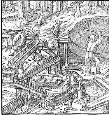
A—TROUGH. B—WOODEN SHOVEL. C—TUB. D—LAUNDER. E—WOODEN TROWEL. F—TRANSVERSE TROUGH. G—PLUG. H—FALLING WATER. I—DITCH. K—BARROW CONVEYING MATERIAL TO BE WASHED. L—PICK LIKE THE BEAK OF A DUCK WITH WHICH THE MINER DIGS OUT THE MATERIAL FROM WHICH THE SMALL STONES ARE OBTAINED.
