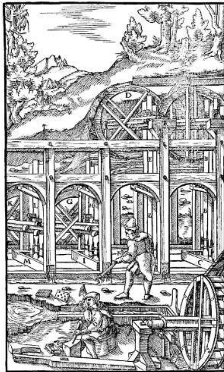
A—FIRST MACHINE. B—ITS STAMPS. C— ITS MORTAR-BOX. D—SECOND MACHINE. E —ITS STAMPS. F—ITS MORTAR-BOX. G— THIRD MACHINE. H—ITS STAMPS. I—ITS MORTAR-BOX. K—FOURTH MACHINE. L—ITS STAMPS. M—ITS MORTAR-BOX. [Pg 320]
