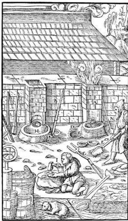
A, B—TWO FURNACES. C—FOREHEARTH. D—DIPPING-POTS. THE MASTER STANDS AT THE ONE FURNACE AND DRAWS AWAY THE SLAGS WITH AN IRON FORK. E—IRON FORK. F—WOODEN HOE WITH WHICH THE CAKES OF MELTED PYRITES ARE DRAWN OUT. G— THE FOREHEARTH CRUCIBLE: ONE-HALF INSIDE IS TO BE SEEN OPEN IN THE OTHER FURNACE. H—THE HALF OUTSIDE THE FURNACE. I—THE ASSISTANT PREPARES THE FOREHEARTH, WHICH IS SEPARATED FROM THE FURNACE THAT IT MAY BE SEEN. K— BAR. L—WOODEN RAMMER. M—LADDER. N—LADLE. [Pg 387]
