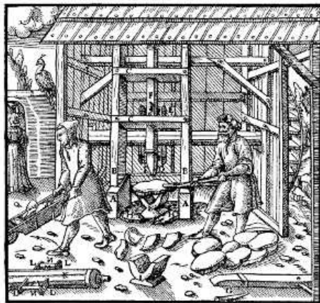
A—BLOCK OF WOOD. B—UPRIGHT POSTS. C—TRANSVERSE BEAMS. D—HEAD OF THE STAMP. E—ITS TOOTH. F—THE HOLE IN THE STAMP-STEM. G—IRON BAR. H—MASSES OF LEAD. I—THE BRONZE SADDLE. K—AXLE. L—ITS ARMS. M—LITTLE IRON AXLE. N—BRONZE PIPE. [Pg 501]
