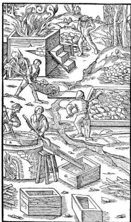
A—FURNACE. B—ENCLOSED SPACE. C—ALUMINOUS ROCK. D—DEEP LADLE. E—CALDRON. F—LAUNDER. G—TROUGHS. [Pg 571]
