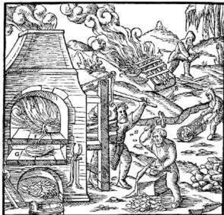
A—WOOD. B—BRICKS. C—PANS. D—FURNACE. E—CRUCIBLE. F—PIPE. G—DIPPING-POT. [Pg 435]
