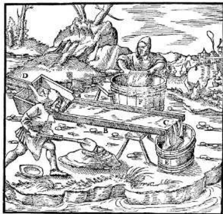
A—HEAD OF FRAME. B—FRAME. C—CLOTH. D—SMALL LAUNDER. E—TUB SET BELOW THE FRAME. F—TUB IN WHICH CLOTH IS WASHED. [Pg 331]
