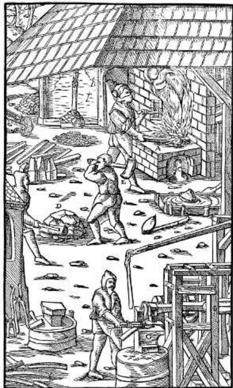
A—HEARTH. B—HEAP. C—SLAG-VENT. D—IRON MASS. E—WOODEN MALLET. F—HAMMER. G—ANVIL. [Pg 422]
