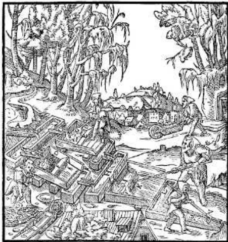
A—LAUNDER. B—CROSS TROUGH. C—TWO SPOUTS. D—BOXES. E—PLATE. F— GRATING. G—SHOVELS. H—SECOND CROSS TROUGH. I—STRAKE. K—WOODEN SCRUBBER. L—THIRD CROSS TROUGH. M— LAUNDER. N—THREE-TOOTHED RAKE. [Pg 345]
