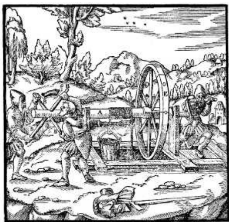
A—BARREL. B—STRAIGHT LEVERS. C—USUAL CRANK. D—SPOKES OF WHEEL. E—RIM OF THE SAME WHEEL. [Pg 162]
