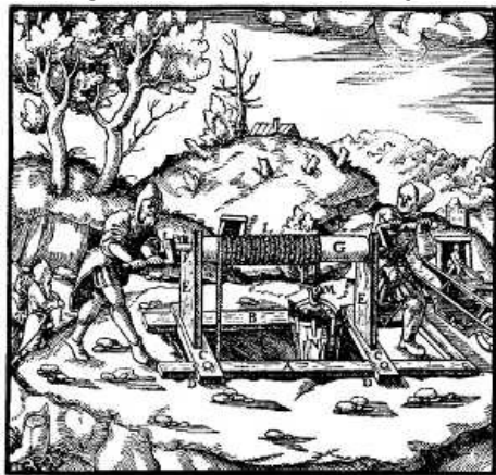
A—TIMBER PLACED IN FRONT OF THE SHAFT. B—TIMBER PLACED AT THE BACK OF THE SHAFT. C—POINTED STAKES. D—CROSS-TIMBERS. E—POSTS OR THICK PLANKS. F—IRON SOCKETS. G—BARREL. H—ENDS OF BARREL. I—PIECES OF WOOD. K—HANDLE. L—DRAWING-ROPE. M—ITS HOOK. N—BUCKET. O—BALE OF THE BUCKET. [Pg 161]
