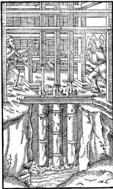
A—TAPPETS OF PISTON-RODS. B—CAMS OF THE BARREL. C—SQUARE UPPER PARTS OF PISTON-RODS. D—LOWER ROUNDED PARTS OF PISTON-RODS. E—CROSS-BEAMS. F—PIPES. G—APERTURES OF PIPES. H—TROUGH. (Fifth kind of pump—see p. 181 ). [Pg 182]
