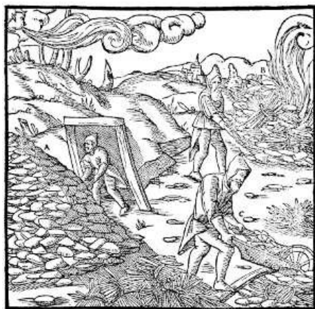
A—HEAP OF CUPRIFEROUS STONES. B—KINDLED HEAP. C—STONES BEING TAKEN TO THE BEDS OF FAGGOTS. [Pg 278]
