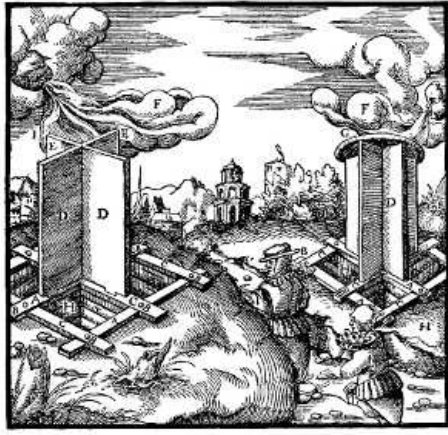
A—SILLS. B—POINTED STAKES. C— CROSS-BEAMS. D—UPRIGHT PLANKS. E— HOLLOWES. F—WINDS. G—COVERING DISC. H—SHAFTS. I—MACHINE WITHOUT A COVERING. [Pg 201]
