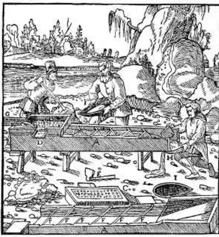
A—SLUICE. B—BOX. C—BOTTOM OF INVERTED BOX. D—OPEN PART OF IT. E—IRON HOE. F—RIFFLES. G—SMALL LAUNDER. H—BOWL WITH WHICH SETTLEINGS ARE TAKEN AWAY. I—BLACK BOWL IN WHICH THEY ARE WASHED. [Pg 323]
