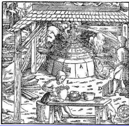
A—FURNACE. B—STICKS OF WOOD. C—LITHARGE. D—PLATE. E—THE FOREMAN WHEN HUNGRY EATS BUTTER, THAT THE POISON WHICH THE CRUCIBLE EXHALES MAY NOT HARM HIM, FOR THIS IS A SPECIAL REMEDY AGAINST THAT POISON. [Pg 474]
