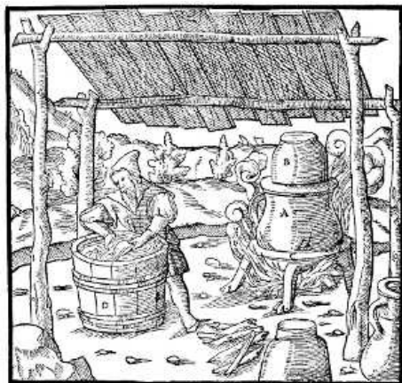
A—LARGER POT. B—SMALLER. C—TRIPOD. D—TUB IN WHICH THE SAND IS WASHED. [Pg 431]
