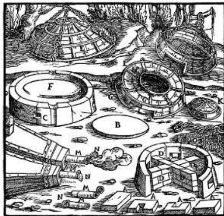
A—RECTANGULAR STONES. B—SOLE-STONE. C—AIR-HOLES. D—INTERNAL WALLS. E—DOME. F—CRUCIBLE. G—BANDS. H—BARS. I—APERTURES IN THE DOME. K—LID OF THE DOME. L—RINGS. M—PIPES. N—VALVES. O—CHAINS. [Pg 468]
