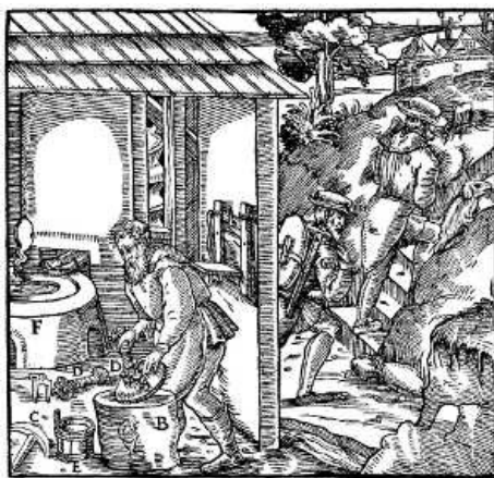
A—CAKE. B—STONE. C—HAMMER. D—BRASS WIRE. E—BUCKET CONTAINING WATER. F—FURNACE FROM WHICH THE CAKE HAS BEEN TAKEN, WHICH IS STILL SMOKING. G—LABOURER CARRYING A CAKE OUT OF THE WORKS. [Pg 476]
