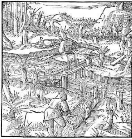
A—RIVER. B—WEIR. C—GATE. D—AREA. E—MEADOW. F—FENCE. G—DITCH. [Pg 318]
