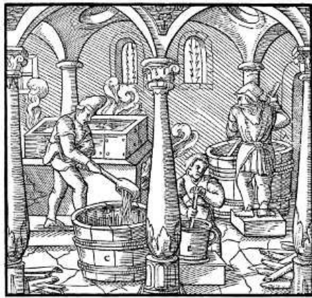
A—VAT IN WHICH THE SODA IS MIXED. B— CALDRON. C—TUB IN WHICH CHRYSOCOLLA IS CONDENSED. D—COPPER WIRES. E— MORTAR. [Pg 561]
