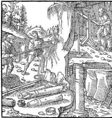
A—ERECT TIMBER. B—AXLE. C—SWEEP WHICH TURNS ABOUT THE AXLE. D—PISTON ROD. E—CROSS-BAR. F—RING WITH WHICH TWO PIPES ARE GENERALLY JOINED. [Pg 178]
