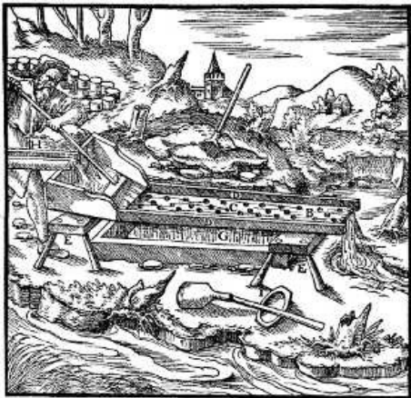
A—HEAD OF FRAME. B—FRAME. C—HOLES. D—EDGE-BOARDS. E—STOOLS. F—SCRUBBER. G—TROUGH. H—LAUNDER. I—BOWL. [Pg 322]
