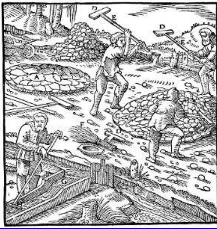
A—AREA PAVED WITH STONES. B—BROKEN ORE. C—AREA COVERED WITH BROKEN ORE. D—IRON TOOL. E—ITS HANDLE. F—BROOM. G—SHORT STRAKE. H—WOODEN HOE. [Pg 272]
