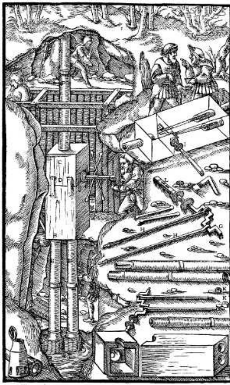
A—Box. B—LOWER PART OF BOX. C—UPPER PART OF SAME. D—CLAMPS. E—PIPES BELOW THE BOX. F—COLUMN PIPE FIXED ABOVE THE BOX. G—IRON AXLE. H—PISTON-RODS. I—WASHERS TO PROTECT THE BEARINGS. K—LEATHERS. L—EYES IN THE AXLE. M—RODS WHOSE ENDS ARE WEIGHTED WITH LUMPS OF LEAD. N—CRANK. ( This plate is unlettered in the first edition but corrected in those later. ) [Pg 180]
