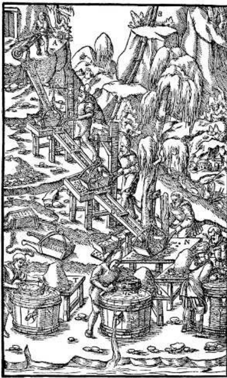
A—WORKMAN CARRYING BROKEN ROCK IN A BARROW. B—FIRST CHUTE. C—FIRST BOX. D—ITS HANDLES. E—ITS BALES. F—ROPE. G—BEAM. H—POST. I—SECOND CHUTE. K—SECOND BOX. L—THIRD CHUTE. M—THIRD BOX. N—FIRST TABLE. O—FIRST SIEVE. P—FIRST TUB. Q—SECOND TABLE. R—SECOND SIEVE. S—SECOND TUB. T—THIRD TABLE. V—THIRD SIEVE. X—THIRD TUB. Y—PLUGS. [Pg 291]
