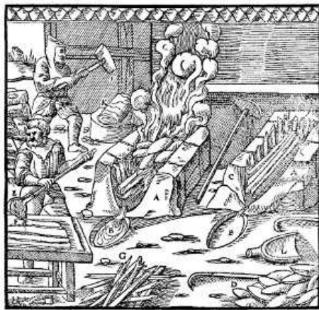
A—HEARHS. B—DIPPING-POTS. C—WOOD. D—CAKES. E—LADLE. F—COPPER PLATE. G—LATTICE-SHAPED BARS. H—IRON DIES. I—WOODEN MALLET. K—MASS OF TIN BARS. L—SHOVEL. [Pg 418]
