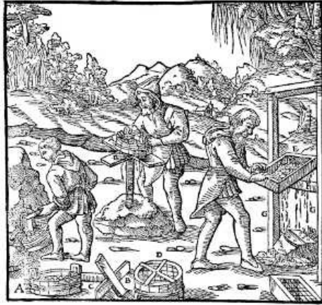
A—SIEVE. B—SMALL PLANKS. C—POST. D— —BOTTOM OF SIEVE. E—OPEN BOX. F— SMALL CROSS-BEAM. G—UPRIGHT POSTS. [Pg 288]
