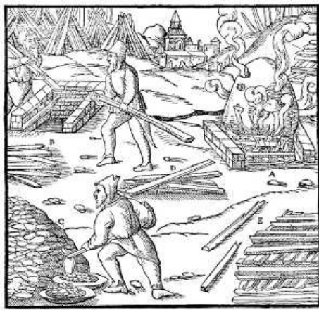
A—LIGHTED PYRE. B—PYRE WHICH IS BEING CONSTRUCTED. C—ORE. D—WOOD. E—PILE OF THE SAME WOOD. [Pg 275]
