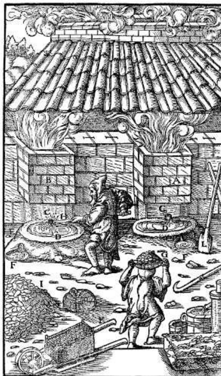
A, B—TWO FURNACES. C—TAP-HOLES OF FURNACES. D—FOREHEARTHS. E—THEIR TAP-HOLES. F—DIPPING-POTS. G—AT THE ONE FURNACE STANDS THE SMELTER CARRYING A WICKER BASKET FULL OF CHARCOAL. AT THE OTHER FURNACE STANDS
