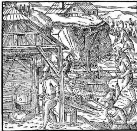
A—BOX. B—BALE. C—ROPE. D—BEAM. E—HANDLES. F—FIVE-TOOTHED RAKE. G— —SIEVE. H—ITS HANDLES. I—POLE. K— ROPE. L—TIMBER. [Pg 289]
