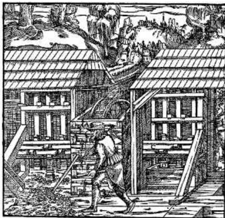
A—Box. ALTHOUGH THE UPPER PART IS NOT OPEN, IT IS SHOWN OPEN HERE, THAT THE WHEEL MAY BE SEEN. B—WHEEL. C—CAM-SHAFT. D—STAMPS. [Pg 286]
