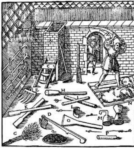
A—FURNACE. B—LADDER. C—BOARD FIXED TO IT. D—HOE. E—FIVE-TOOTHED RAKE. F—WOODEN SPATULA. G—BROOM. H—RAMMER. I—RAMMER, SAME DIAMETER. K—TWO WOODEN SPATULAS. L—CURVED BLADE. M—BRONZE RAMMER. N— ANOTHER BRONZE RAMMER. O—WIDE SPATULA. P—ROD. Q—WICKER BASKET. R —TWO BUCKETS OF LEATHER IN WHICH WATER IS CARRIED FOR PUTTING OUT A CONFLAGRATION, SHOULD THE OFFICINA CATCH FIRE. S—BRASS PUMP WITH WHICH THE WATER IS SQUIRTED OUT. T—TWO HOOKS. V—RAKE. X—WORKMAN BEATING THE CLAY WITH AN IRON IMPLEMENT. [Pg 377]
