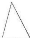
A TRIANGLE HAVING ALL ITS ANGLES ACUTE AND ITS THREE SIDES UNEQUAL. [Pg 137]
