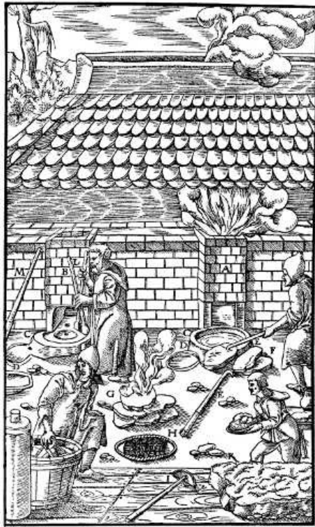
A, B—TWO FURNACES. C—FOREHEARTH. D—DIPPING-POT. THE SMELTER STANDING BY THE FIRST FURNACE DRAWS OFF THE SLUGS WITH A HOOKED BAR. E—HOOKED BAR. F—SLUGS. G—THE ASSISTANT DRAWING A BUCKET OF WATER WHICH HE POURS OVER THE GLOWING SLUGS TO QUENCH THEM. H—BASKET MADE OF TWIGS OF WOOD INTERTWINED. I—RABBLE. K—ORE TO BE SMELTED. L—THE MASTER STANDS AT THE OTHER FURNACE AND PREPARES THE FOREHEARTH BY RAMMING IT WITH TWO RAMMERS. M—CROWBAR. [Pg 385]
