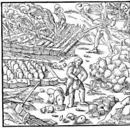
A—HEARTH. B—POLES. C—HEARTH WITHOUT FIRE IN WHICH THE POTS ARE PLACED. D—ROCKS. E—ROWS OF POTS. F—UPPER POTS. G—LOWER POTS. [Pg 427]
