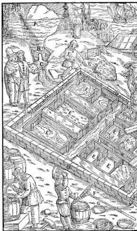
A—SEA. B—POOL. C—GATE. D—TRENCHES. E—SALT BASINS. F—RAKE. G—SHOVEL. [Pg 547]
