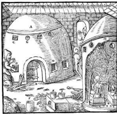
A—ENCLOSED CHAMBER. B—DOOR. C—LITTLE WINDOWS. D—MOUTHS THROUGH THE WALLS. E—FURNACE IN THE ENCLOSED CHAMBER. F—POTS. [Pg 430]
