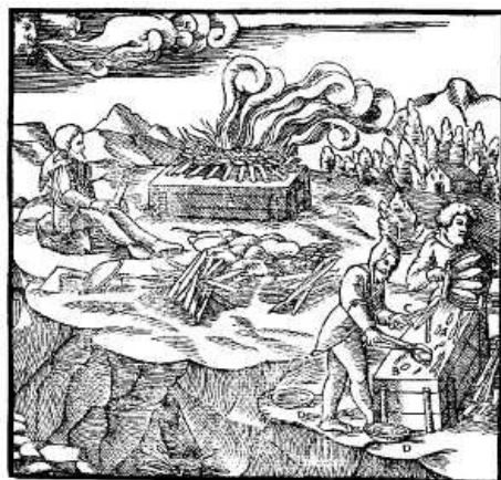
A—HEARTH IN WHICH ORE IS MELTED. B—HEARTH ON WHICH LIE DROPS OF BISMUTH.
