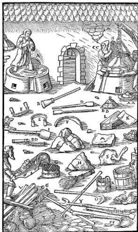
A—AN ARTIFICER TAMPING THE CRUCIBLE WITH A RAMMER. B—LARGE RAMMER. C—BROOM. D—TWO SMALLER RAMMERS. E—CURVED IRON PLATES. F—PART OF A WOODEN STRIP. G—SIEVE. H—ASHES. I—IRON SHOVEL. K—IRON PLATE. L—BLOCK OF WOOD. M—ROCK. N—BASKET MADE OF WOVEN TWIGS. O—HOOKED BAR. P—SECOND HOOKED BAR. Q—OLD LINEN RAG. R—BUCKET. S—DOESKIN. T—BUNDLES OF STRAW. V—WOOD. X—CAKES OF LEAD ALLOY. Y—FORK. Z—ANOTHER WORKMAN COVERS THE OUTSIDE OF THE FURNACE WITH LUTE WHERE THE DOME FITS ON IT. AA—BASKET FULL OF ASHES. BB—LID OF THE DOME. CC—THE ASSISTANT STANDING ON THE STEPS POURS CHARCOAL INTO THE CRUCIBLE THROUGH THE HOLE AT THE TOP OF THE DOME. DD—IRON IMPLEMENT WITH WHICH THE LUTE IS BEATEN. EE—LUTE. FF—LADLE WITH WHICH THE WORKMAN OR MASTER TAKES A SAMPLE. GG—RABBLE WITH WHICH THE SCUM OF IMPURE LEAD IS DRAWN OFF. HH—IRON WEDGE WITH WHICH THE SILVER MASS IS RAISED. [Pg 470]
