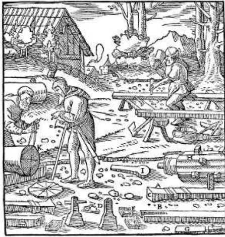
A—STAMP. B—STEM CUT OUT IN LOWER PART. C—SHOE. D—THE OTHER SHOE, BARBED AND GROOVED. E—QUADRANGULAR IRON BAND. F—WEDGE. G—TAPPET. H—ANGULAR CAM-SHAFT. I—CAMs. K—PAIR OF COMPASSES. [Pg 285]
