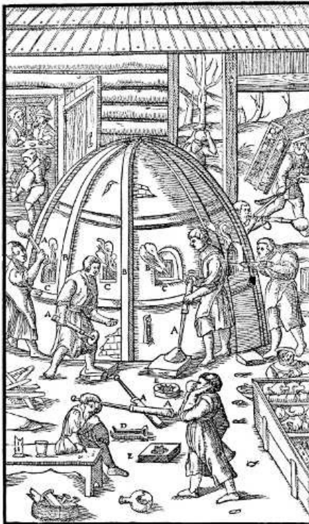
A—BLOW-PIPE. B—LITTLE WINDOW. C—MARBLE. D—FORCEPS. E—MOULDS BY MEANS OF WHICH THE SHAPES ARE PRODUCED. [Pg 591]
