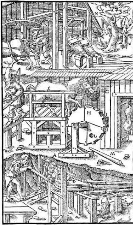
A—MACHINE FIRST DESCRIBED. B—THIS WORKMAN, TREADING WITH HIS FEET, IS COMPRESSING THE BELLOWS. C—BELLOWS WITHOUT NOZZLES. D—HOLE BY WHICH HEAVY VAPOURS OR BLASTS ARE BLOWN OUT. E—CONDUITS. F—TUNNEL. G—SECOND MACHINE DESCRIBED. H—WOODEN WHEEL. I—ITS STEPS. K—BARS. L—HOLE IN SAME WHEEL. M—POLE. N—THIRD MACHINE DESCRIBED. O—UPRIGHT AXLE. P—ITS TOOTHED DRUM. Q—HORIZONTAL AXLE. R—ITS DRUM WHICH IS MADE OF RUNDLES. [Pg 211]
