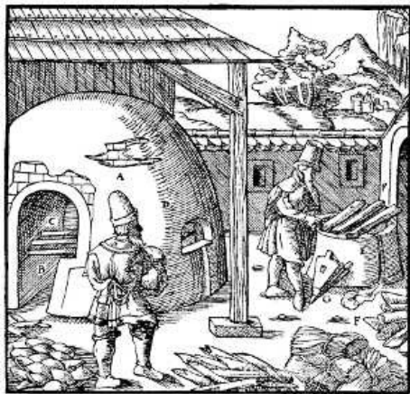
A—FURNACE SIMILAR TO AN OVEN. B—PASSAGE. C—IRON BARS. D—HOLE THROUGH WHICH THE LITHARGE IS DRAWN OUT. E—CRUCIBLE WHICH LACKS A DOME. F—THICK STICKS. G—BELLOWS. [Pg 482]
