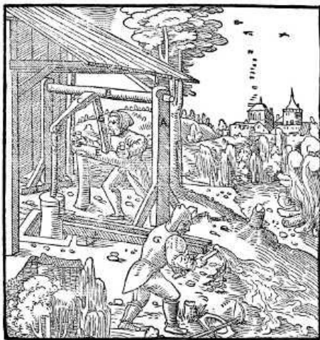
A—POSTS. B—AXLE. C—WOODEN BARS. D—PISTON ROD. E—SHORT PIECE OF WOOD. F—DRAIN. G—THIS MAN IS DIVERTING THE WATER WHICH IS FLOWING OUT OF THE DRAIN, TO PREVENT IT FROM FLOWING INTO THE TRENCHES WHICH ARE BEING DUG. [Pg 179]
