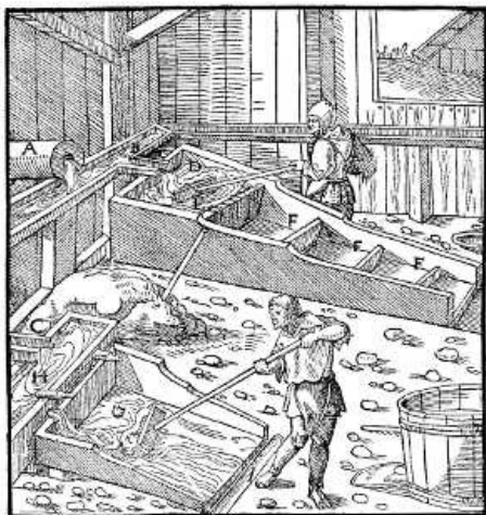
A—PIPE. B—CROSS LAUNDER. C—SMALL TROUGHS. D—HEAD OF THE BUDDLE. E—WOODEN SCRUBBER. F—DIVIDING BOARDS. G—SHORT STRAKE. [Pg 302]
