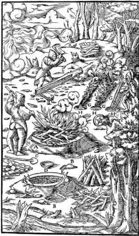
A—PIT ACROSS WHICH WOOD IS PLACED. B—FOREHEARTH. C—LADLE. D—IRON MOULD. E—CAKES. F—EMPTY POT LINED WITH STONES IN LAYERS. G—TROUGH. H—PITS DUG AT THE FOOT OF THE TROUGH. I—SMALL WOOD LAID OVER THE TROUGH. K—WIND. [Pg 434]
