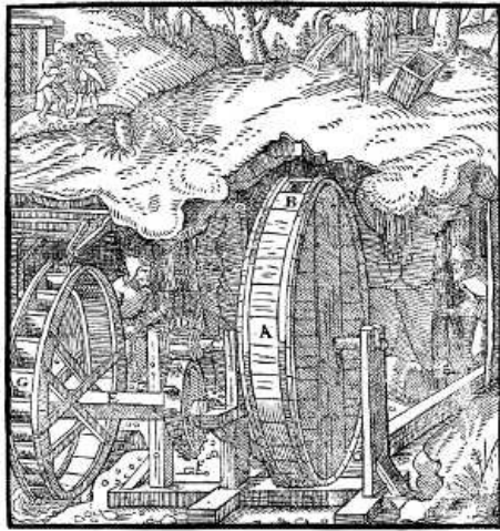
A—HOLLOW DRUM. B—ITS BLOW-HOLE. C— —AXLE WITH FANS. D—DRUM WHICH IS MADE OF RUNDLES. E—LOWER AXLE. F— ITS TOOTHED WHEEL. G—WATER WHEEL. [Pg 206]
