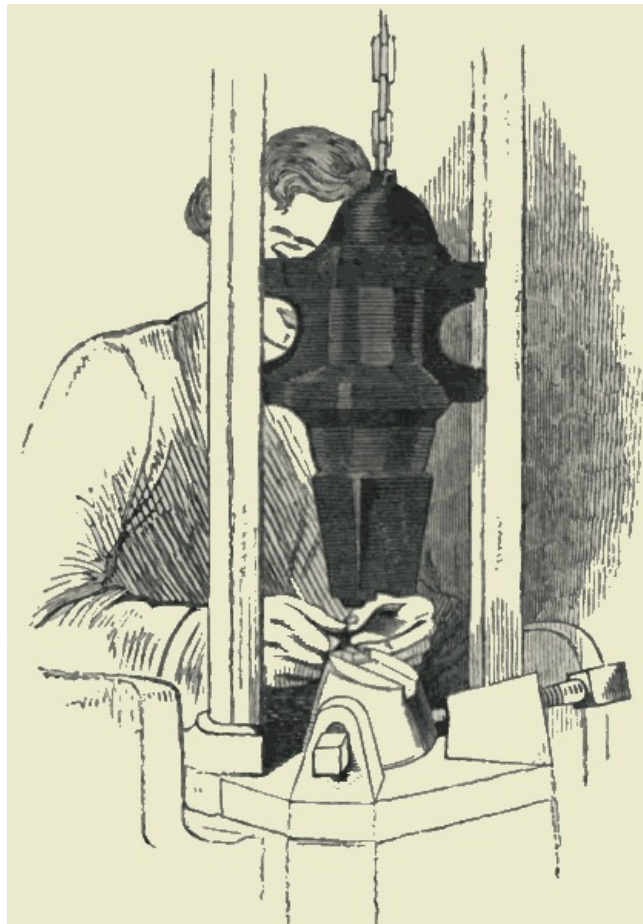
Stamping the eye of a needle.
