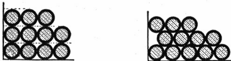
FIGS. 242 and 243.—Square and hexagonal order of "bedding." The term bedding is an expression used to indicate the relation between the cross sectional area of the winding when wound square, as in fig. 242, and when wound in some other way, as in fig. 243. In the square order of bedding, the degree of bedding equals zero.
