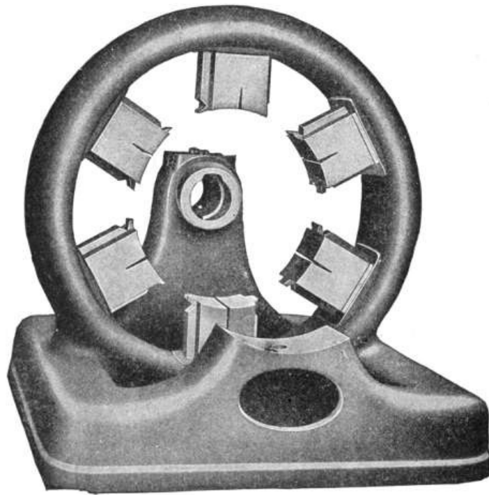
FIG. 236.—Fort Wayne one piece frame with cast welded combined cores and pole pieces. In any electrical apparatus a magnetic circuit of low reluctance requires less energy to maintain a given flux than one having a comparatively high reluctance. To reduce this to a minimum the pole pieces and cores are combined into one part and then cast welded into the yoke or frame. Thus the continuity of the magnetic circuit is practically unbroken save for the air gap.
