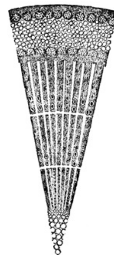
SECTION OF WOOD. MAGNIFIED 50 DIAMETERS.
