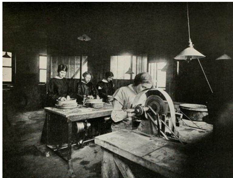
SLITTING AND ROUGHING OPTICAL GLASS
