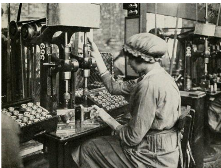
DRILLING SAFETY-PIN HOLE IN FUSE
