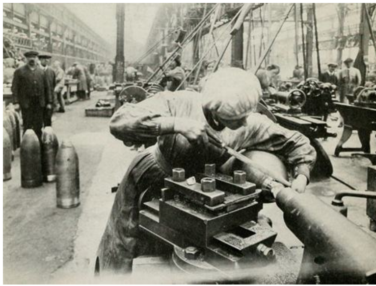
TURNING THE OUTSIDE AND FORMING THE NOSE-END OF A 9.2-INCH HIGH-EXPLOSIVE SHELL
