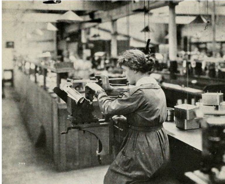
ENGRAVING METAL PARTS FOR COMPASSES
