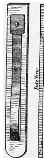
FIG. 2.—Free Reed Vibrator, Mason & Hamlin American Organ.
