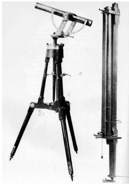
Figure 10.—Transit and equal-altitude instrument (left) made by Ellicott in 1789 and used by him in the survey of the boundary between the United States and Florida and in other surveys. USNM 152080.
