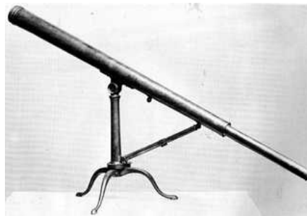
Figure 73.—Telescope used by Andrew Ellicott for his survey of the boundary between the United States and the Spanish territory of Florida. The instrument is signed "W. & S. Jones, 135 Holborn, London." USNM 152082.
