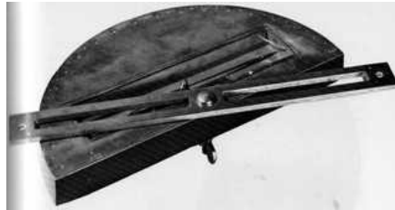
Figure 34.—18th-century semicircumferentor. Inscribed brass plate is mounted on a mahogany block; brass sighting bars are mounted on a swivelling bar. The trough compass is on a silvered dial. In collection of the writer.
