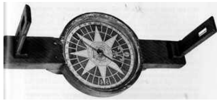
Figure 41.—Wooden surveying compass made by James Halsy (1695-1767) of Boston. The instrument is 11 in. long. In collection of East India Marine Hall, Peabody Museum, Salem, Massachusetts.
