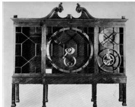
Figure 7.—Orrery built by David Rittenhouse for the University of Pennsylvania. The center section shows the motions of the planets and their satellites and the right-hand section the eclipses of the Sun and Moon. The case, considered to be an outstanding example of colonial cabinet-work, was made by John Folwell.
