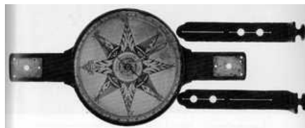
Figure 8.—Brass surveying compass inscribed "Made by Benjamin Rittenhouse, 1787." Photo courtesy Ohio State Museum, Columbus, Ohio.
