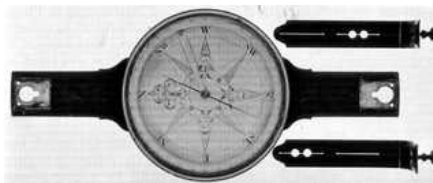
Figure 29.—Brass surveying compass made by Isaac Chandlee (1760-1813) of Nottingham, Maryland. Photo courtesy Ohio State Museum.
