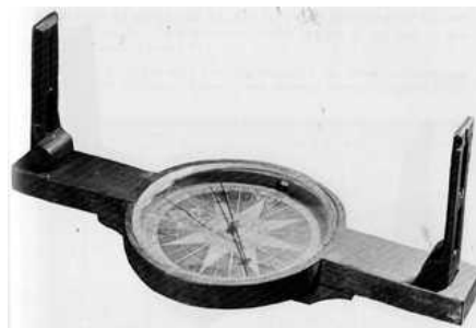
Figure 43.—Wooden surveying compass, made and sold by Thomas Greenough. The instrument is made of gumwood and has a paper compass card; it is 13-1/4 in. long and has a diameter of 5-3/4 in. In collection of Franklin Institute, Philadelphia.
