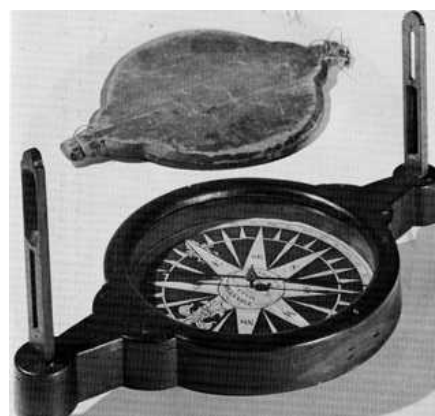
Figure 52.—Mahogany surveying compass made by Samuel Thaxter of Boston. Length, 13 in.; diameter, 7-1/2 in. Wooden frame slides off to permit removal of glass and adjustment of needle. Sighting bars are of boxwood. In collection of the writer.
