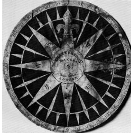
Figure 53.—Compass card from earlier form of wooden surveying compass made by Samuel Thaxter of Boston. From an instrument in the collection of the writer.
