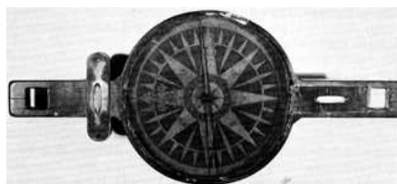
Figure 67.—Wooden surveying compass made by Thomas Salter Bowles of Portsmouth, New Hampshire. With spirit level. Made of birch, the compass is 13 in. long and has a diameter of 6 in. In the Streeter Collection of Weights and Measures, Yale University.
