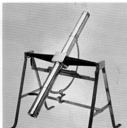
Figure 3.—Transit telescope made by David Rittenhouse and used by him for the observation of the transit of Venus in 1769. Brass, 33-1/2-in. tube on a 25-in. axis, with an aperture of 1-3/4 in. and a focal length of 32 in. Photo courtesy the American Philosophical Society.
