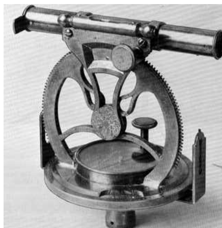
Figure 74.—Theodolite used by Orange Warner Ellis about 1780 for surveying boundary between the United States and Canada in the area which is now Vermont. USNM 309596.
