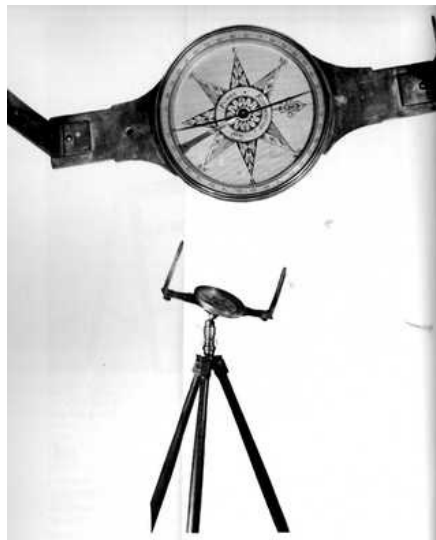
Figure 4.—Surveying compass marked "Potts and Rittenhouse." Believed to be the work of David Rittenhouse in partnership with Thomas Potts. Photo courtesy the American Philosophical Society.
