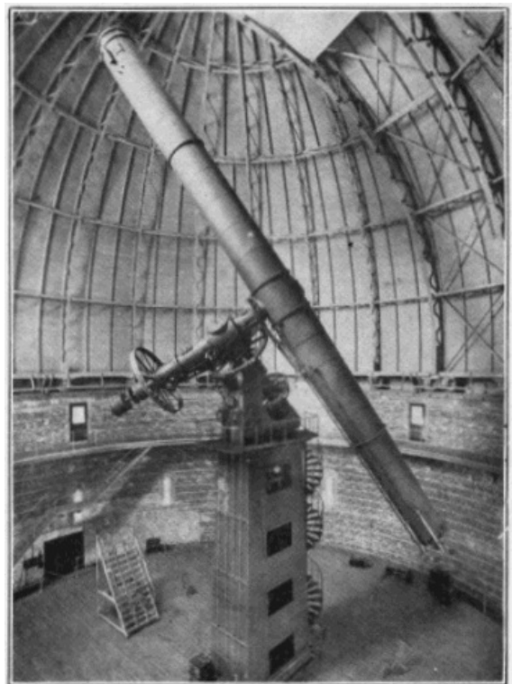
THE LARGEST REFRACTOR, THE 40-INCH TELESCOPE AT YERKES OBSERVATORY. DOME 90 FT. IN DIAMETER. ( Photo, Yerkes Observatory. )
