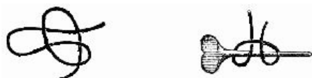
Fig. 28—Loops for attaching to frame hooks. Fig. 29—Loops for taking frame keys.
