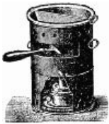
Fig. 1.— Glue-pot for heating by petroleum.
