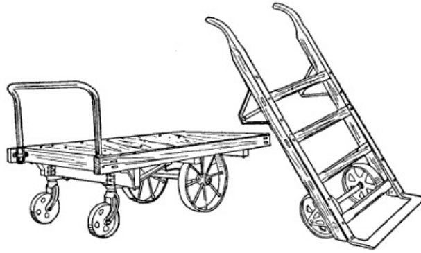
Figure 225.—Barn Trucks. The platform truck is made to move boxed apples and other fruit. The bag truck is well proportioned and strong, but is not full ironed.
