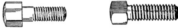
Figure 94.—Machine-Bolt and Set-Screw. The bolt to the left is used to clamp cylinder heads in place. The set-screw to the right is the cup variety. The end is countersunk to form a cup with a sharp rim.
