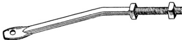
Figure 89.—Wagon-Box Brace. It is offset to hold the rave and to brace the sideboard at the rear and the front ends and sometimes in the middle of light wagon beds.
