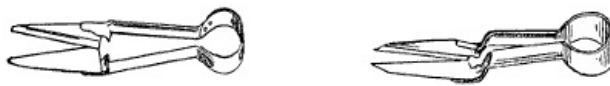
Figure 213.—Shears. The first pair is used for sheep shearing. The second is intended for cutting grass around the edges of walks and flower beds.
