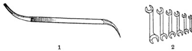
Figure 60.—(1) Cotter Pin Tool. Handy for inserting or removing all sorts of cotter keys. (2) Nest of S Wrenches of different sizes. Farmers have never appreciated the value of light, handy wrenches to fit all sorts of nuts and bolt heads closely.
