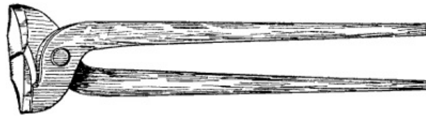
Figure 63.—Cutting Nippers. For cutting the points from horseshoe nails after they are driven through the hoof to hold the shoe in place. These nippers are hard tempered and should not be used for any other purpose.
