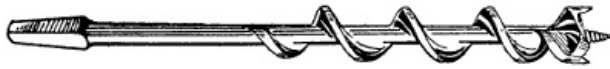
Figure 27.—Auger-Bits. For smooth boring the lip bits are best. The side cutters project beyond the cutting lips to cut the circle ahead of the chips. For boring green wood the single-worm clears better than the double-worm bit.
