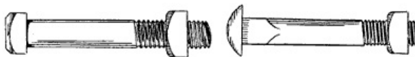
Figure 85.—Machine Bolt and Carriage Bolt. The first is used against iron and the second against wood, but this rule is not arbitrary. The rounded side of the nuts are turned in against wood; the flat side against washers or heavier iron. Use square head bolts if you expect to take them out after the nuts have rusted on.
