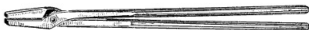
Figure 58.—Blacksmith Tongs. Straight tongs made to hold \frac{3}{8} " iron is the handiest size. Two or three pairs for larger sizes of iron and one pair smaller come in handy.
