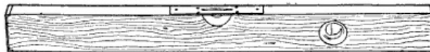
Figure 23.—Carpenter's Level. For practical farm work the level should be 24" or 30" long. Wood is the most satisfactory material. The best levels are made up of different layers of wood glued together to prevent warping or twisting. For this reason a good level should be carefully laid away in a dry place immediately after using.
