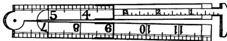
Figure 5.—Caliper Rule. A handy slide caliper shop rule is made with a slide marked in fractions of inches as shown in the drawing. The diameter of a rivet, bolt or other round object may be taken instantly. It is not so accurate as calipers for close measurements, but it is a practical tool for farm use.
