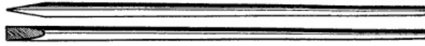
Figure 21.—Handspike. A wooden handspike or pry is about seven feet long by 3 inches thick at the prying end. In the North it is usually made from a hickory or an ironwood or a dogwood sapling. The bark is removed and the handle is worked round and smooth on the shave horse. It is better to cut the poles in the winter when the sap is in the roots. After the handspikes are finished they should be covered deep with straw so they will season slowly to prevent checking.
