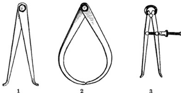
Figure 57.—Calipers: (1) A pair of tight-joint inside calipers. (2) Its mate for taking outside dimensions. (3) A pair of spring-jointed, screw-adjustment inside calipers for machinists' use.
