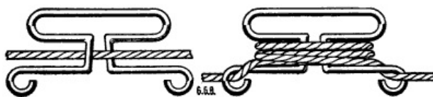
Figure 229.—Clothes Line Tightener. This device is made of No. 9 wire bent as shown in the illustration.
