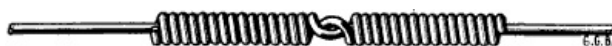
Figure 74.—Wire Splice. With a little practice wire may be wound close enough to prevent slipping.
