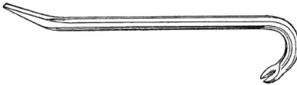
Figure 22.—Wrecking Bar for pulling nails and to pry broken parts from other wreckage.
