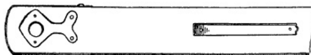
Figure 73.—Showing how to fit the irons on the forward end of a wagon reach.
