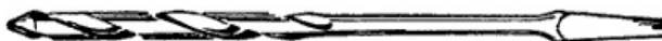
Figure 25.—Wood-Boring Twist Drill Bit. Twist drills for wood have longer points than drills for boring iron.
