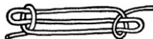
Figure 206.—Sheepshank, two half hitches in a rope to take up slack. The rope may be folded upon itself as many times as necessary.
