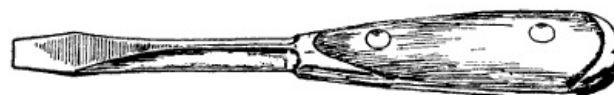
Figure 19.—Heavy Screwdriver. The strongest and cheapest screwdriver is made from a single bar of steel. The wooden handle is made in two parts and riveted as shown.
