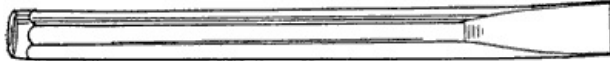
Figure 46.—Cold-Chisel. There are more flat cold-chisels than all other shapes. They are easily made in the farm shop and it is good practice. They are usually made from octagon steel. Different sizes are needed according to the work in hand. A piece of \frac{3}{8} " steel 6" long makes a handy cold-chisel for repair work.
