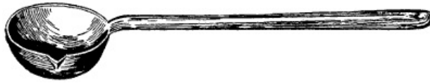
Figure 98.—Melting Ladle. Babbitting shaft boxing requires a melting ladle. It should be about five inches across the bowl and about three inches deep. That is a good size to heat in a forge fire.
