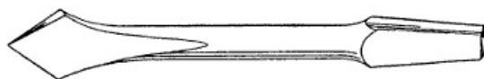
Figure 54.—Countersink. This is the old style, blacksmith-made, flat countersink. It will do quick work but not so smooth as the fluted kind.
