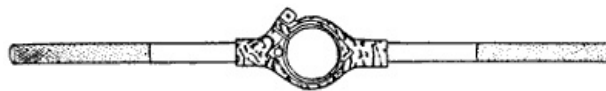
Figure 82.—Stock for Round Dies. The opening is turned true and sized accurately to fit. The screw applies pressure to hold the die by friction.
