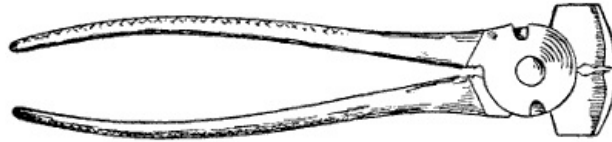
Figure 194.—Fence Pliers. This is a heavy fence tool made to pull fence staples and to stretch, cut and splice wire.
