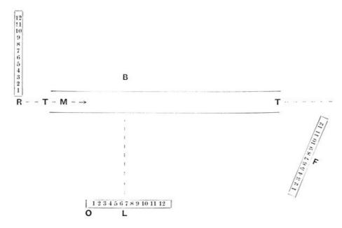
TT represents the track along which the model M was caused to move. B is the background, divided into spaces of 5 centimetres square for the purpose of measurement.
