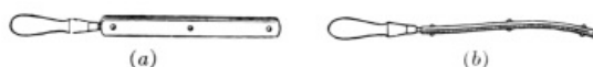
FIG. 2 (a) represents a straight bar made of a strip of brass and a strip of iron riveted together and attached to a handle. Upon heating the compound bar in a gas flame, the brass expands faster than the iron causing the bar to bend toward the latter as in Fig. 2 (b).
