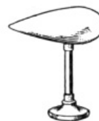
FIG. 202.—More charge at the pointed end.
