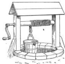
FIG. 91.—Windlass used in drawing water from a well.
