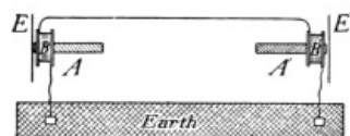
FIG. 309.—The simplest telephone system. It consists of two telephone receivers connected in series on a circuit. It will work, but not satisfactorily.
