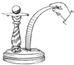
FIG. 59.—The ball remains when the card is driven away.
