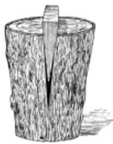
FIG. 102.—One use of the wedge.
