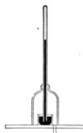
FIG. 32.—The mercury drops as the air is removed.
