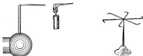
FIG. 203.—Electrical wind produced by a pointed conductor.
