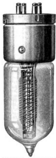
FIG. 427.—Vacuum tube, receiving type. (Western Electric Co.)
