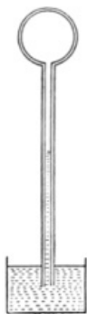
FIG. 1.—When the bulb is heated, the air within expands forcing down the water in the tube.
