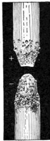
FIG. 276.—The appearance of a pair of used carbons.
