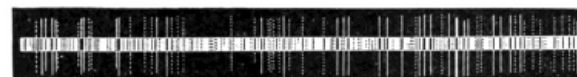
FIG. 408.—The bright line spectrum of iron and its coincidences with some of the dark lines of the solar spectrum.
