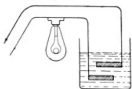
FIG. 264.—The current passes only when ions are present in the liquid.
