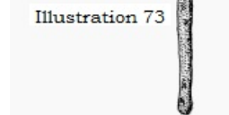
Illustration 71.—Series of wrought-iron flooring nails and brads. One-half. Illustration 72.—Fragment of clouting nail. Same size. Illustration 73.—Hand-forged spike. One-half. (USNM 59.1811.)
