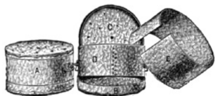
FIG. 44.—Wilson press hoop. A, complete hoop; B, bottom cover with wide flange; C, top cover with narrow flange; D, closed body; E, bandager.
