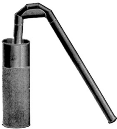
FIG. 36.—Whey siphon with strainer.
