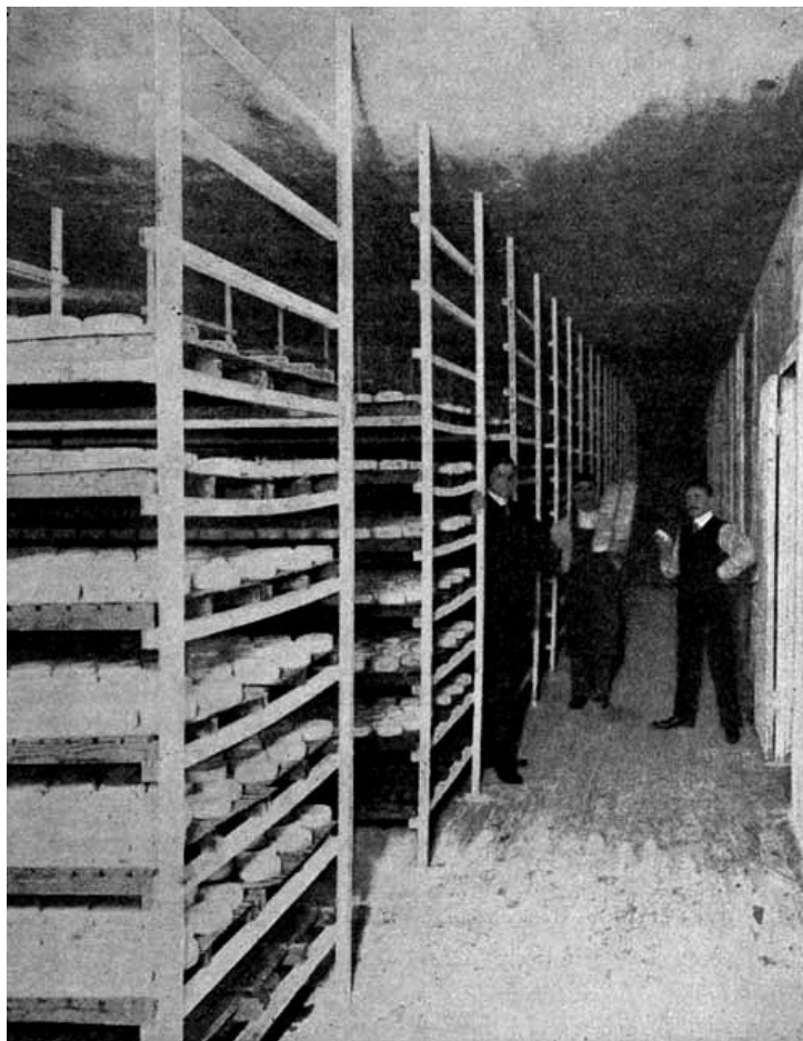
FIG. 20.—Halloir, the first ripening room for Camembert in an American factory.
