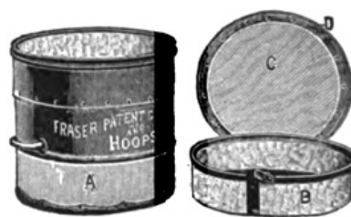
FIG. 45.—Fraser press hoop. A, complete hoop; B, bandager; C, follower; D, fibrous press ring.
