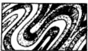
FIG. 174. Folds with Layers thickened at the Crest and thinned along the Limbs
