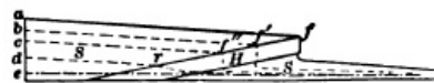
FIG. 57. Diagram illustrating Migration of a Fall due to a Hard Layer H , in the Midst of Soft Layers S and S' , all dipping upstream
