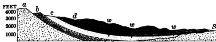
FIG. 29. Section across South Dakota from the Black Hills to Sioux Falls (S), Illustrating the Conditions of Artesian Wells
