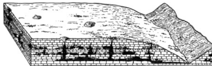
FIG. 30. Diagram of Caverns and Sink Holes
