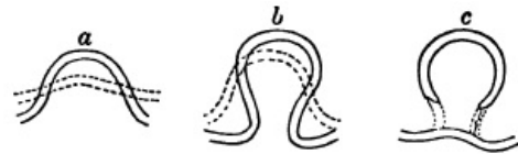
FIG. 76. Development of a Meander The dotted line in a , b , and c shows the stage preceding that indicated by the unbroken line
