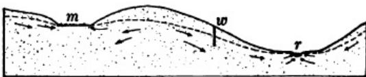
FIG. 24. Diagram Illustrating the Relation of the Ground-Water Surface to the Surface of the Ground
