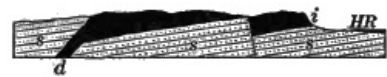
FIG. 243. Diagram of the Palisades of the Hudson i, intrusive sheet; s, sandstone; d, feeding dike; HR, Hudson River
