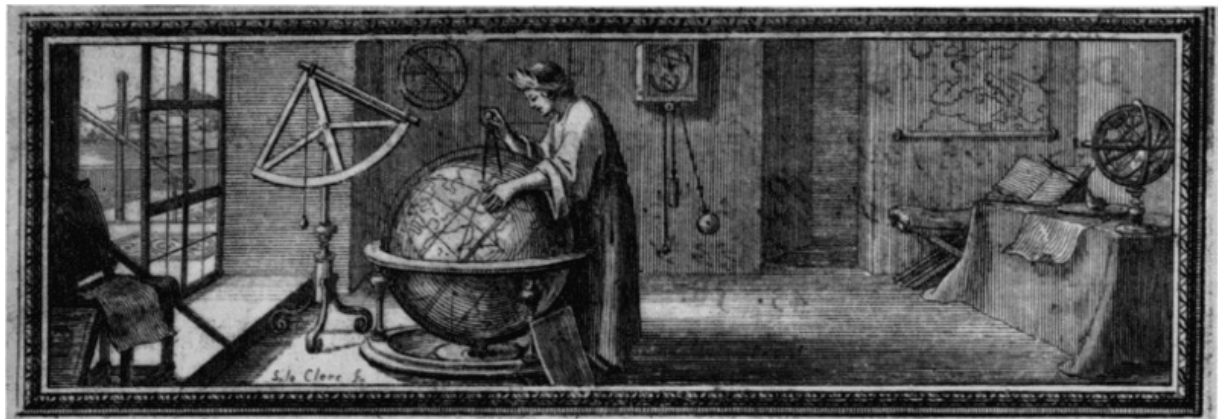
Figure 2.—THIS DRAWING, FROM RICHER'S Observations astronomiques et physiques faites en l'isle de Caienne (Paris, 1679), shows most of the astronomical instruments used by Richer, namely, one of the two pendulum clocks made by Thuret, the 20-foot and the 5-foot telescopes and the large quadrant. The figure may be intended as a portrait of Richer. This drawing was done by Sebastian Le Clerc, a young illustrator who made many illustrations of the early work of the Paris Academy.
