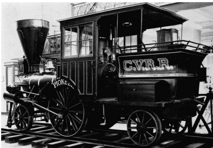
Figure 29.—“PIONEER” on exhibit in old Arts and Industries building, showing the tank and backhead. (Smithsonian photo 48069E.)
