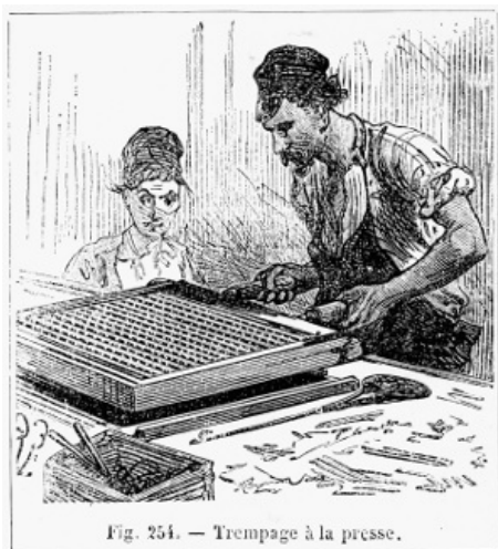
Figure 11.—DIPPING OF MATCHSTICKS in France, about 1870. The frame which holds the matches so that one end protrudes at the bottom, is lowered over a pan containing molten sulfur. The sulfur-covered matches are then dropped into a phosphorous paste. See figure 12 . (From FIGUIER, Merveilles de l'industrie , volume 3, 1874, page 575.)
