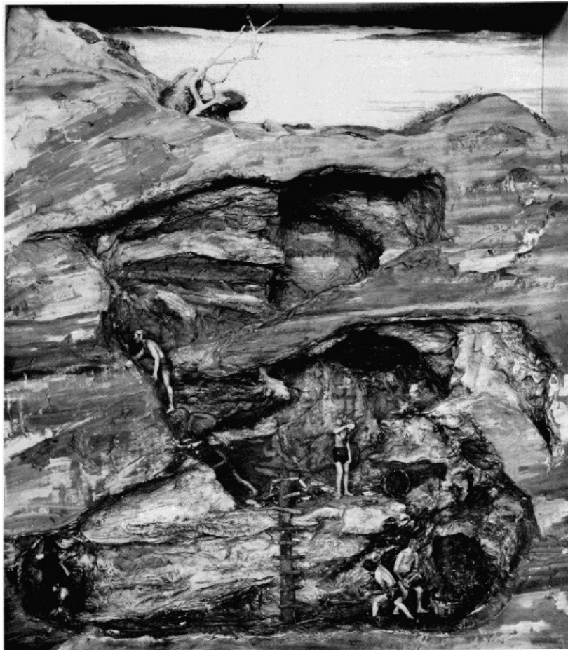
Figure 1.—MINING BY EARLY EUROPEAN CIVILIZATIONS, using fire setting and hand chiseling to break out ore and rock. MHT model— \frac{3}{4} " scale. (Smithsonian photo 49260-H.)
