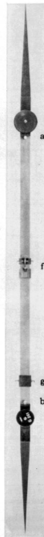
Figure 11.—THE ATTEMPT TO APPROXIMATE the simple (theoretical) pendulum in gravity experiments ended in 1817-18 when Henry Kater invented the compound convertible pendulum, from which the equivalent simple pendulum could be obtained according to the method of Huygens (see text, p. 314). Developed in connection with a project to fix the standard of English measure, Kater's pendulum was called "compound" because it was a solid bar rather than the fine wire or string with which earlier experimenters had tried to approximate a "weightless" rod. It was called convertible because it is alternately swung from the two knife edges ( a and b ) at opposite ends. The weights ( f and g ) are adjusted so that the period of the pendulum is the same from either knife edge. The distance between the two knife edges is then equal to the length of the equivalent simple pendulum.
