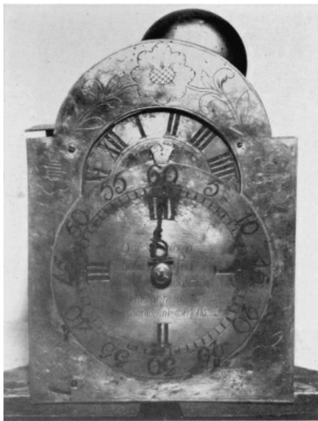
Figure 34.—DIAL PLATE of a brass lantern clock made by Bertolla at the age of 80. (Courtesy of Museo Nazionale della Scienza e della Tecnica, Milan.)
