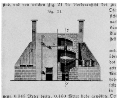
Figure 2.—GALLEY-OVEN, 1869. The picture is a cross section through the front of the oven showing one of the 36 retorts, the receivers for the distillate, and the space in the upper story used for evaporating the mixture of acid solution of calcium phosphate and coal. (According to ANSELME PAYEN, Précis de Chimie industrielle , Paris, 1849; reproduced from HUGO FLECK, Die Fabrikation chemischer Produkte aus thierischen Abfällen , Vieweg, Braunschweig, 1862, page 80 of volume 2, 2nd group, of P. BOLLEY'S Handbuch der chemischen Technologie .)
