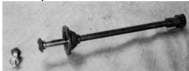
FIGURE 26.—HALF OF JACKSHAFT showing double-shrouded pinion and half of the Columbia differential.
