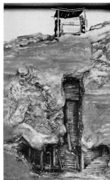
Figure 17.—SOFT-GROUND TUNNELING. The support of walls and roof of mine shaft by simple timbering; 16th century. MHT model— \frac{3}{4} " scale. (Smithsonian photo 49260-J.)
