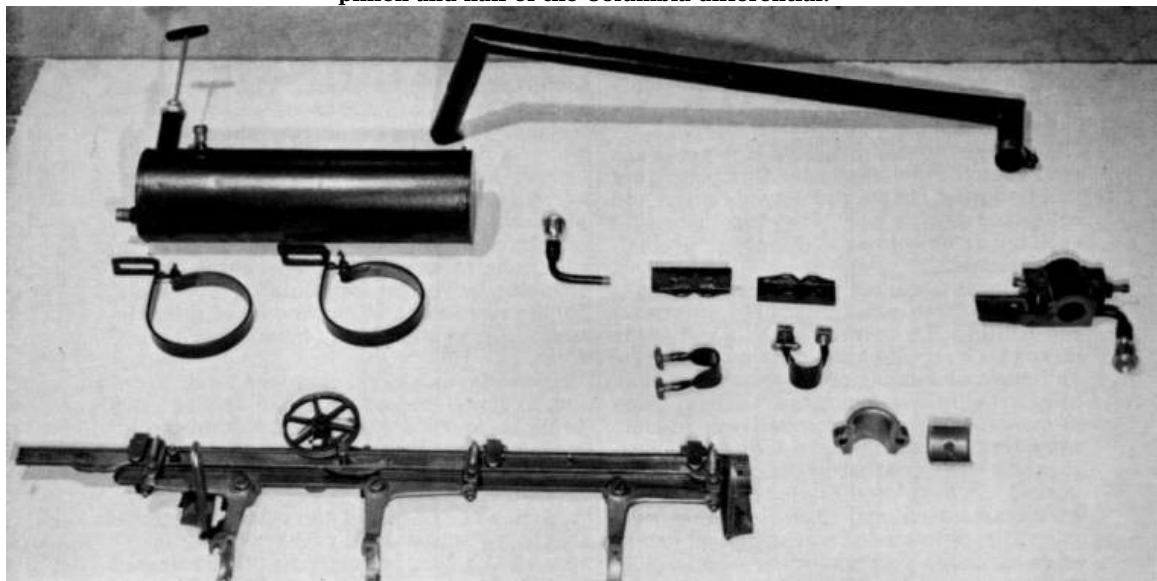
FIGURE 27.—CAM BAR IN FOREGROUND, operated by tiller, actuates the various clutches of the transmission. The overflow gasoline tank with the hand pump can be seen in the rear.
