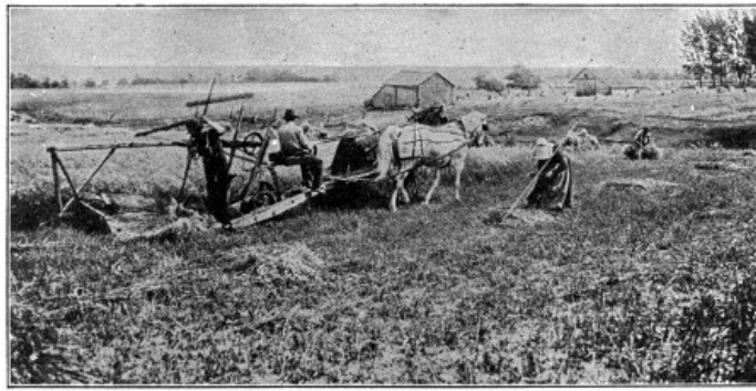
THE MCCORMICK REAPER OF 1845 IN THE FIELD, WITH A SEAT ADDED FOR THE RAKER
