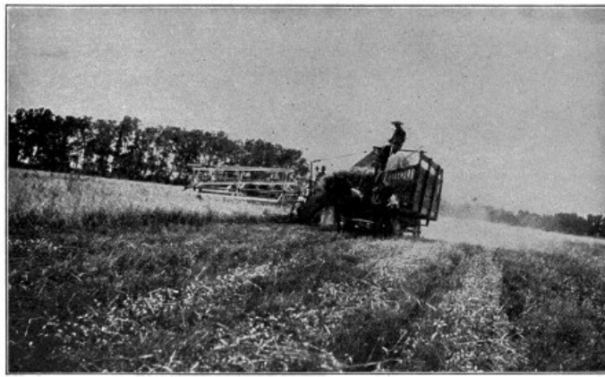
A MCCORMICK HEADER BINDER WHICH ELEVATES THE GRAIN INTO WAGONS WHICH DRIVE ALONGSIDE
