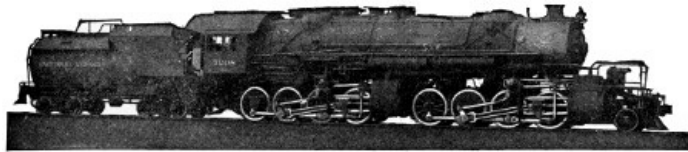
MALLET TYPE FREIGHT LOCOMOTIVE—BALTIMORE & OHIO R. R. Built by American Locomotive Company.
