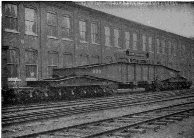
SPECIAL CAR BUILT FOR THE SHIPPING OF LARGE AND HEAVY MATERIAL. [43] (See page 421. )
