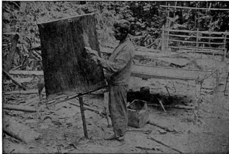
INDIAN WATERPROOFING CLOTH BY "PAINTING" IT WITH RUBBER "MILK"—BRAZIL Courtesy of the United States Rubber Co.
